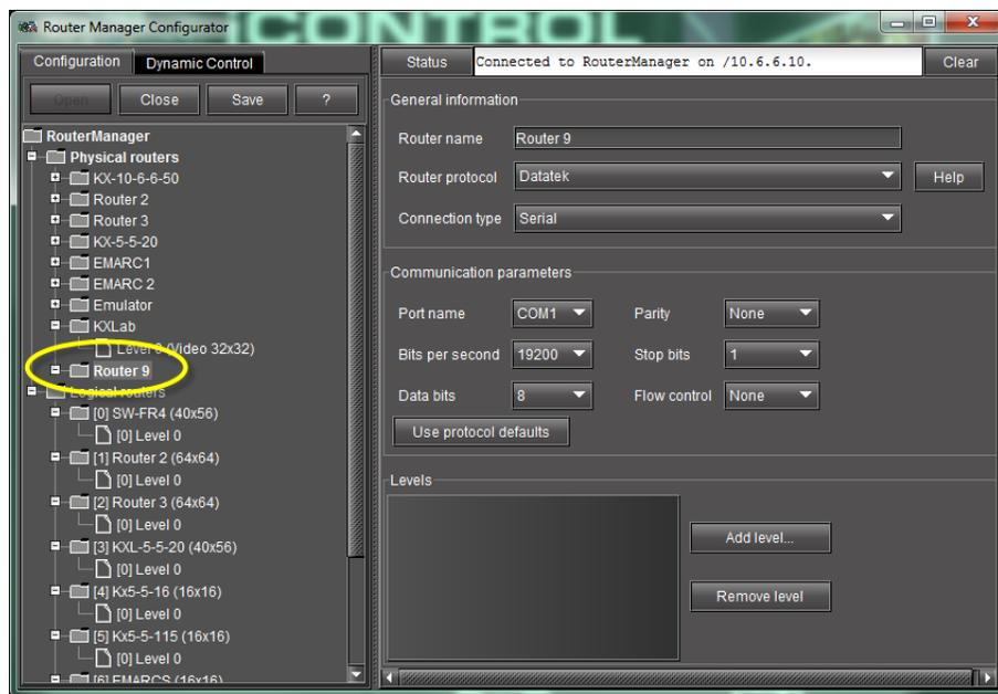
4. Type a name for the router in the **Router name** box.
