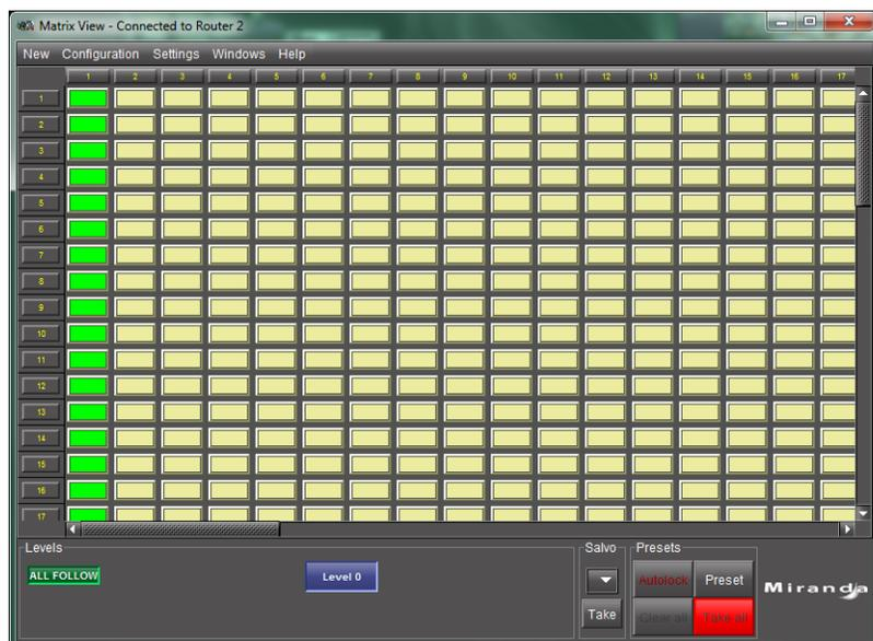
This view is a visual representation of the status for the entire logical router. It displays the complete router status, and allows the configuration of crosspoints to be changed during operation. Three panes at the bottom of the window enable crosspoint operation, in different modes.
