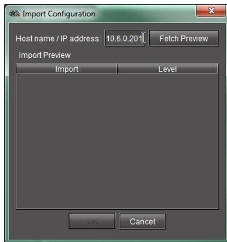
4. In the **Host name / IP address** box, type the host name or IP address of the NVISION router controller whose configuration you would like to import.
