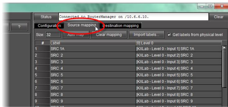
The source mapping table is displayed. The number of rows matches the logical router size that was specified when the logical router was created. The physical devices which serve each level are shown across the top, and the matrix shows which physical input is assigned to each logical input.
