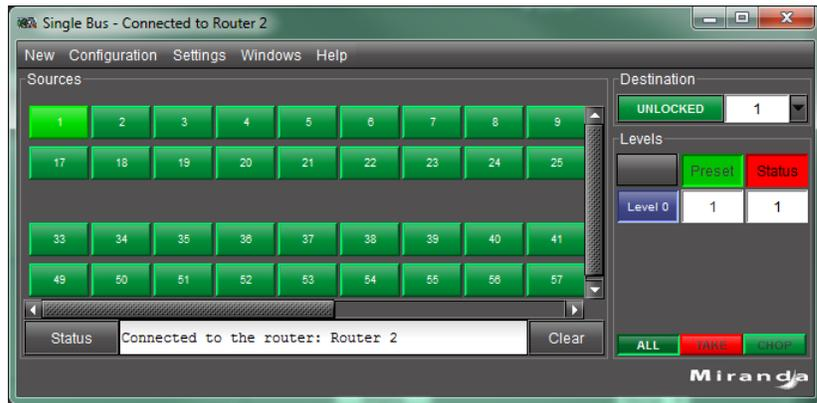
This view enables control of one or more router destinations at the same time. It allows isolates control of one output at a time. Sources appear on the left as a set of buttons, and the destination is on the right.
