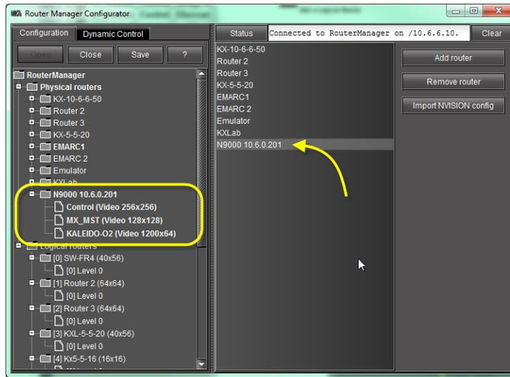
Selecting the physical router in the left pane yields general information, communication parameters, and a list of levels imported from the router.
