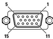
15-pin Sub-D female standard VGA connector
