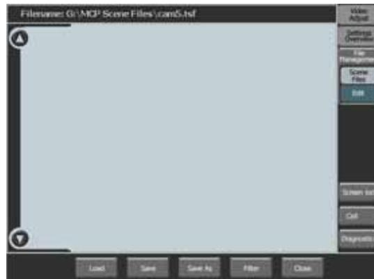
2. Make sure a USB Flash Drive is inserted into the MCP 400. Tap the **Load** button to open the files window. The contents of the root folder of the USB Flash Drive is shown.
