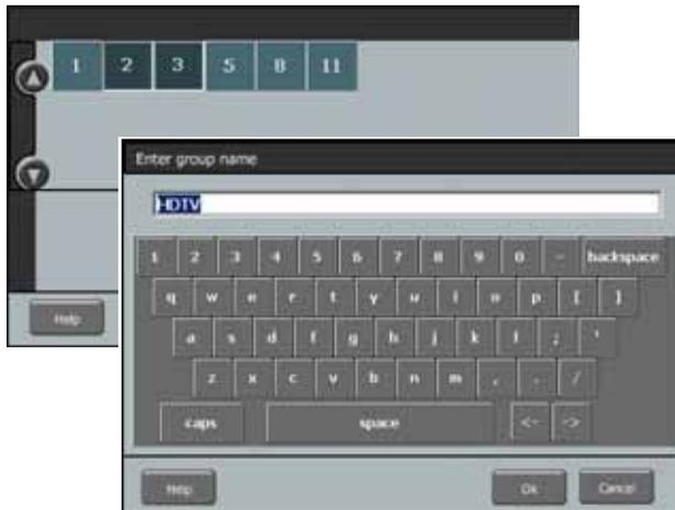
When you are done selecting cameras tap the **OK** button. Use the keyboard layout to enter a name for your new group. Tap the **OK** button to return to the **Options** window. Tap **Close** to return to the camera selection window. The new group has been added to the groups list.
