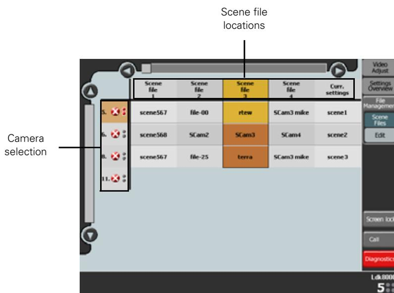
Scene files are stored in scene file locations in the camera or on a USB Flash Drive that is connected to the MCP 400. When the scene files menu is activated, a matrix window is shown. At the top the names of all 7 scene file locations are displayed (scroll to see them all):
