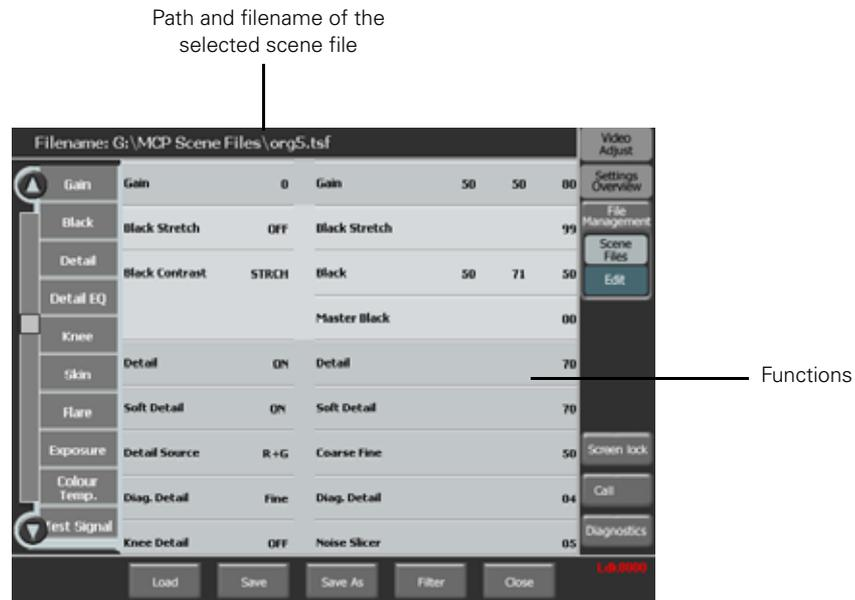
5. Tap the **Filter** button to open the Filter Menu. Select or unselect functions as described in ["Selecting functions" on page 24.](#)
