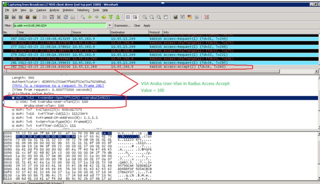
**Figure 46** Configure VSA on a RADIUS Server
