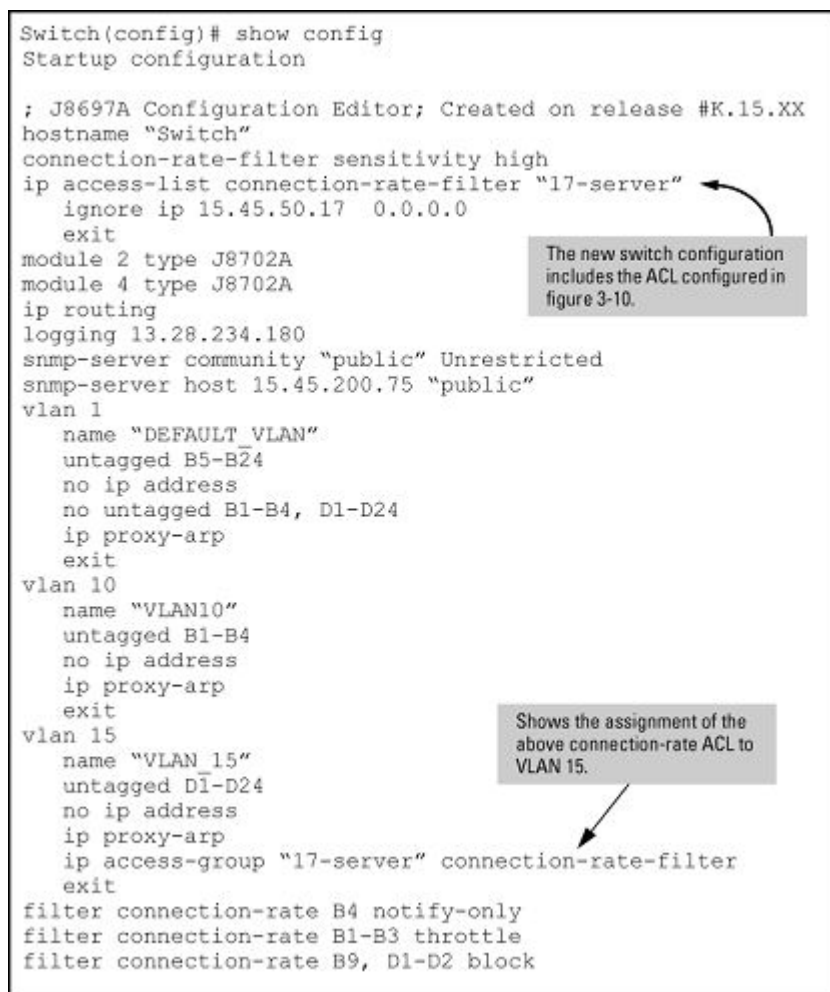
Figure 33: Example of switch configuration display with a connection-rate ACL
