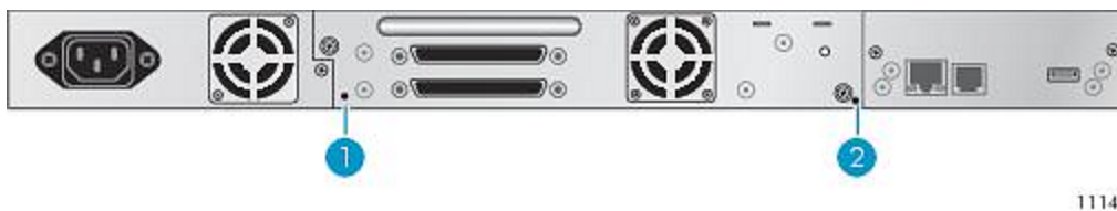
Figure 81 Manual magazine release holes
