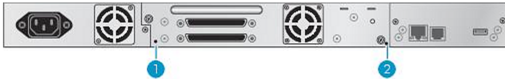
Figure 64 Access holes for the right and left magazine
