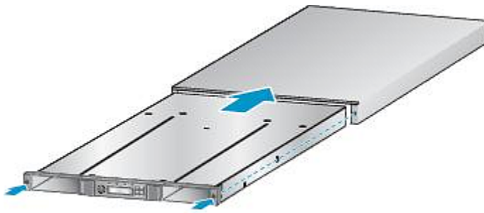
Figure 88 Sliding the Autoloader into the cover
