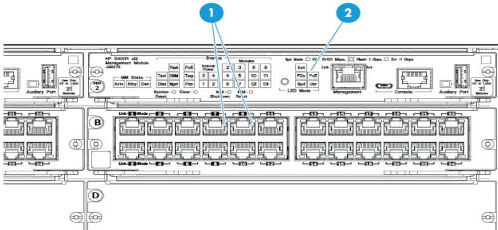
**Figure 1-4. Mode LEDs and LED Mode Select Button**
