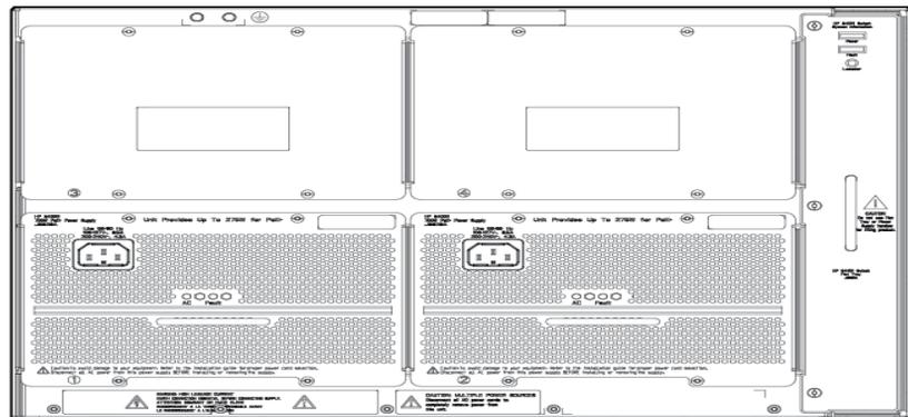
Figure 1-6. Back of a 5412R z12 switch with two power supplies
