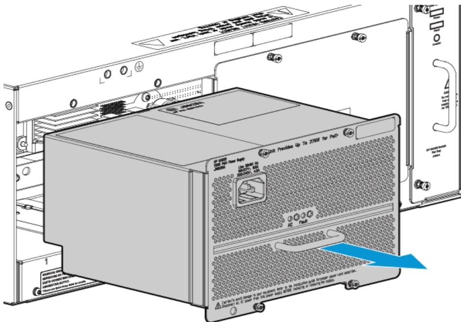
Figure 4-1. Power supply removal
