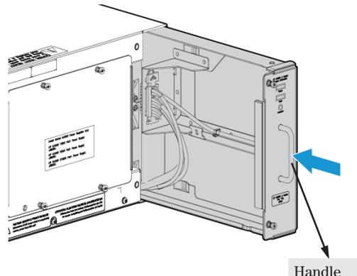
Figure 4-4. 5406R z12 Switch Fan Tray insertion
