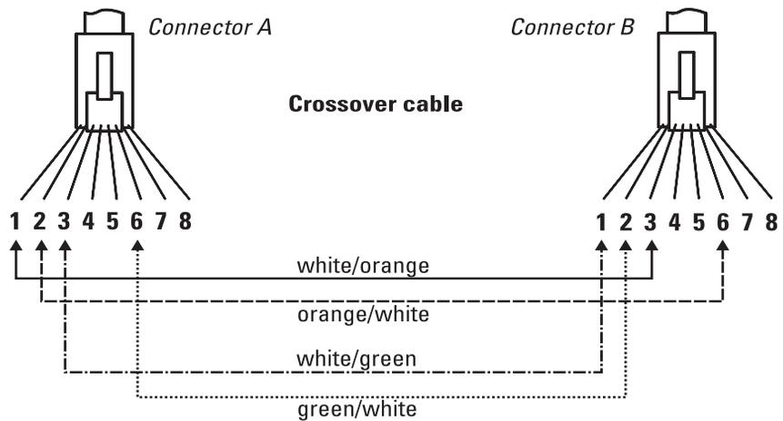
Figure B-3. Cross-over Cable Diagram for 10/100 Mbps Network Connection
