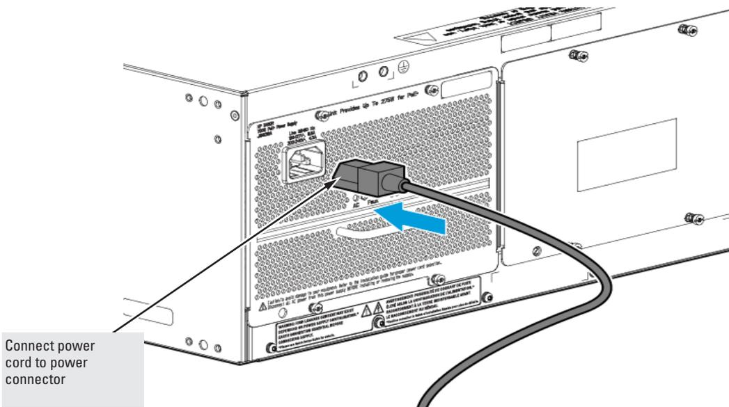
**Figure 2-3. Power connector on back of switch**
