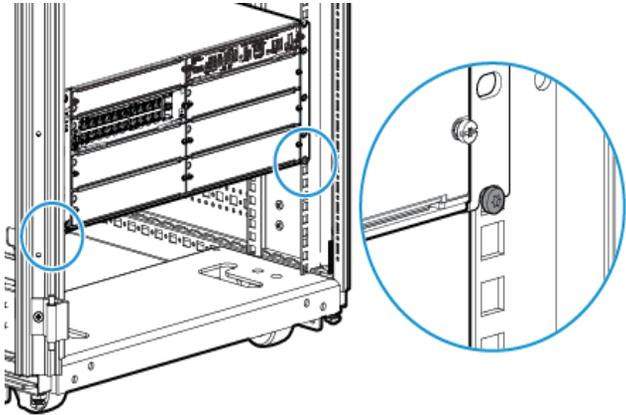
5. Secure the Rack Mount Brackets to the switch with included flat head screws.
