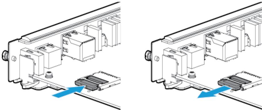
**Figure 4-6. Secure Digital installation and removal**
