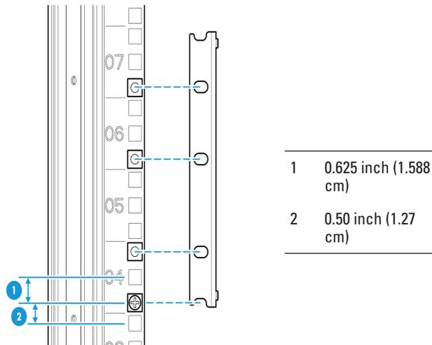
2. Install a screw half-way into this cage nut.
