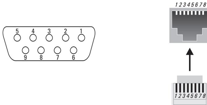
Figure 2-7. RJ-45 to DB-9 pinouts
