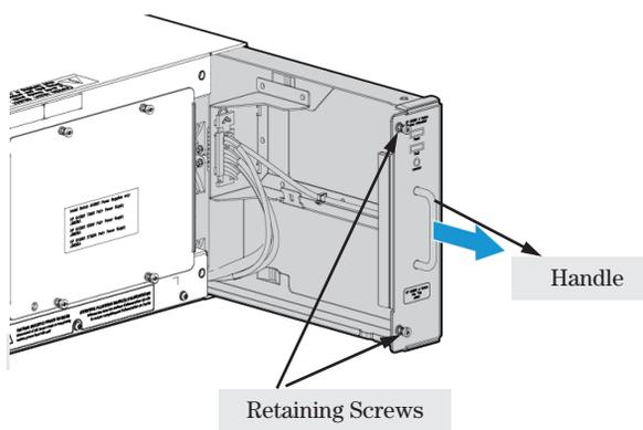
Figure 4-3. 5406R z12 Switch Fan Tray removal
