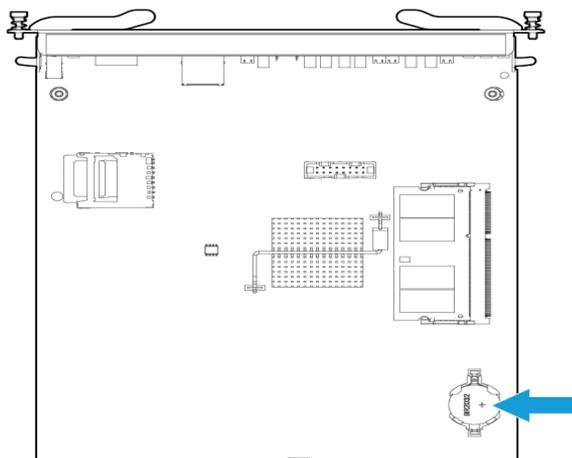
**Figure 2-1. Battery location on Management Module**
