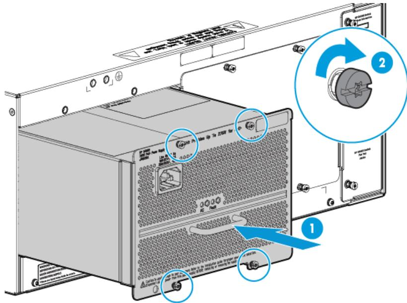
**Figure 2-2. Installing a power supply**
