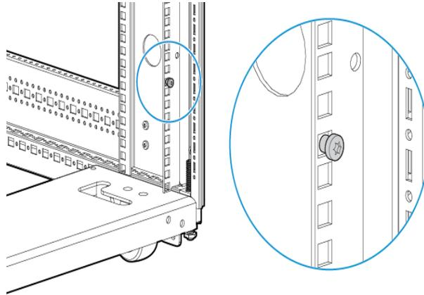
3. Align the included Rack Mount Bracket such that the half-hole lines up with the screw, install additional cage nuts at each hole position in the bracket.
