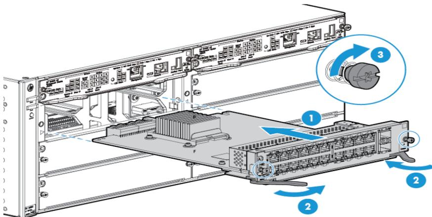
Figure 4-5. Management Module removal and installation
