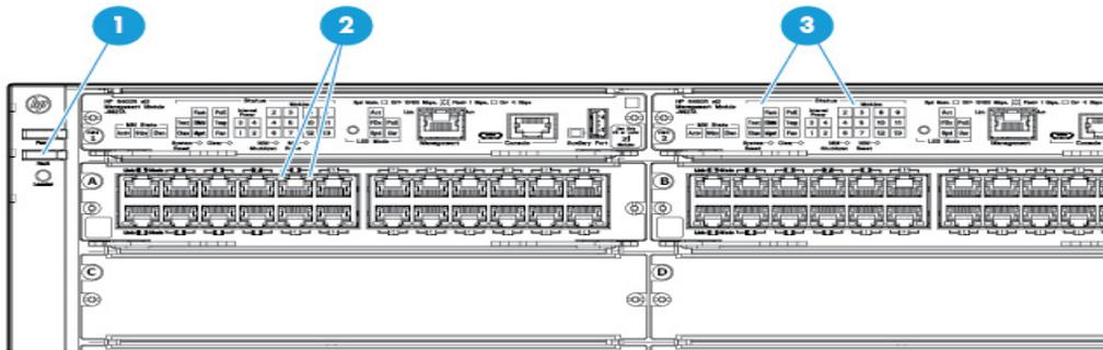
**Figure 2-4. Switch Fault, Module, and Chassis LEDs**
