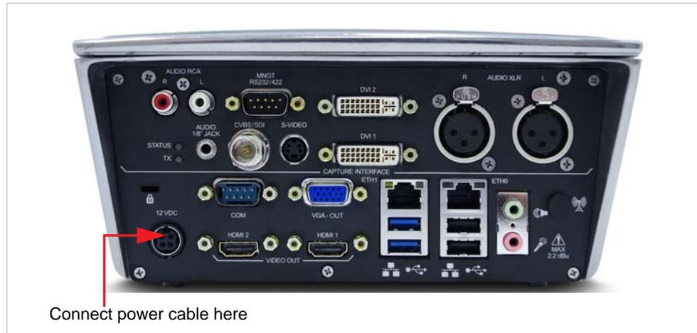
2. Plug the other end of the power cable into a grounded electrical outlet or a separate power source such as an uninterruptible power supply (UPS) or a power distribution unit (PDU).
