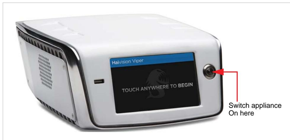
The Power indicator LED should light and you will see the boot progress bar.
