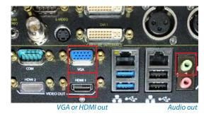
2. (Optional) To set up Audio Talkback or Audio Preview, connect the green Audio Output connector to a speaker. 3. Press the Power button (on the front of the appliance).
