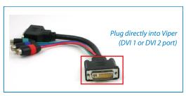
a. Plug the DVI-I male connector on the adaptor directly into either the DVI 1 or DVI 2 input on the Viper.
