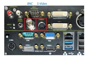
**NOTE:** You can connect multiple video inputs on the Viper and then select the input(s) to use from the Touch Panel interface. This allows you to easily switch between analog and digital video inputs without having to plug and unplug cables.
