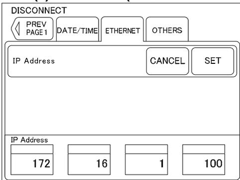
Set the local IP address by the Rotary encoder 1 to 4.
