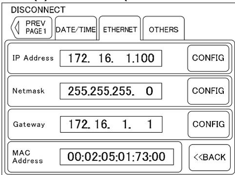
This is the local address information. Press CONFIG button to set the IP Address, the Netmask, and the Gateway. But the TAKEN must be OFF.
