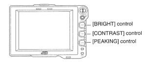
2 Turn the [CONTRAST] control to adjust the contrast of the screen.
