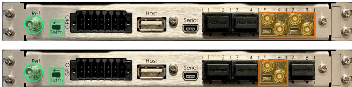
Figure 4-3 MatchBox Generator SFP Rears, SD/HD/3G/4k followed by SD/HD/3G
