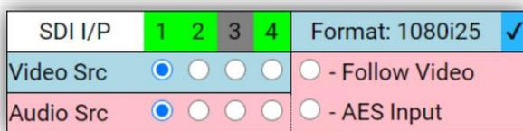
The MatchBox Analyser can analyse audio and video from any of its available SDI inputs, including measuring audio from one input against video from another.
