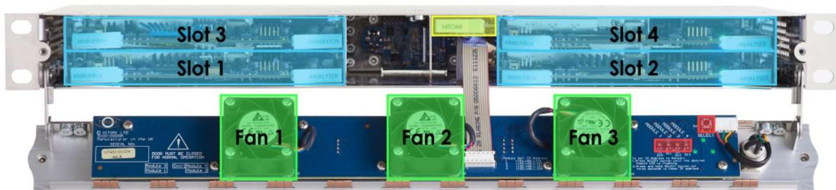
Figure 4-1 - Front view of the xFrame
