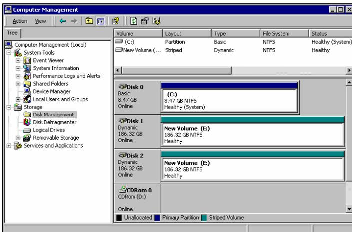
At the completion of format, note the newly prepared disks will have a drive letter associated with it.
