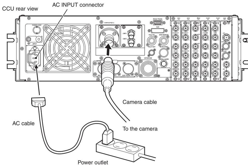
This completes the connection procedure for supplying power from the CCU-890 to the camera. Two methods of power supply to the camera head are available with this configuration.
