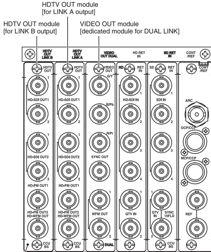
The HDTV OUT module is mounted to the slot for the SDTV OUT module.
