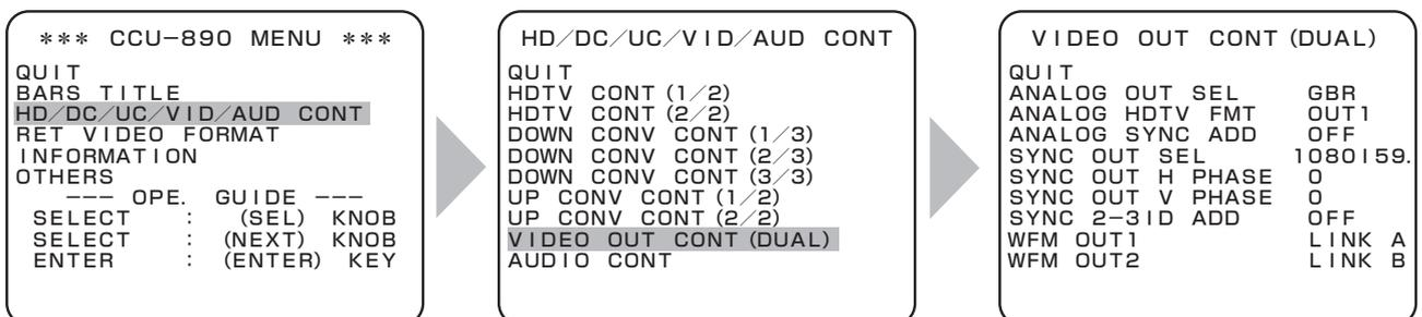
Turn the MASTER PEDESTAL control knob or IRIS control knob to position the flashing cursor on the submenu "HD/DC/UC/VID/AUD CONT," and press the CALL button.
