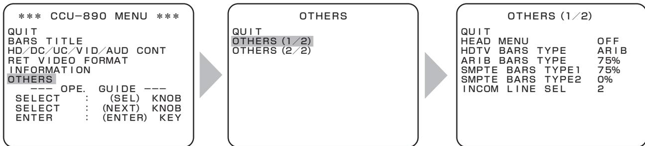
Turn the MASTER PEDESTAL control knob or IRIS control knob to position the flashing cursor on the submenu "OTHERS," and press the CALL button.
