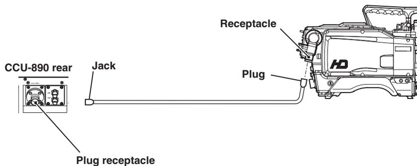
Clean the four sections: receptacle on the camera head, plug receptacle on the CCU, and plug/jack on both ends of the camera cable. The cleaning method for male connectors slightly differs from that for female connectors.
