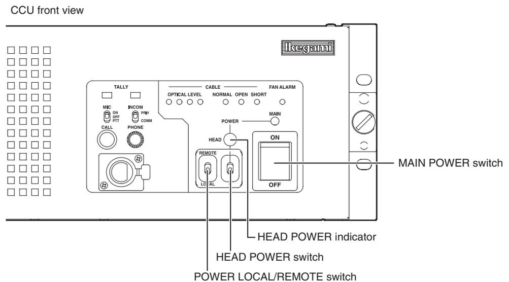
Setting the HEAD POWER switch on the front of the CCU to "ON/OFF" enables control of the power supply to the camera head.
