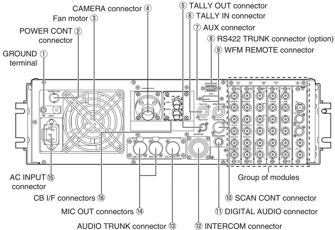
\* Depending on the specification, ⑯ CB I/F connectors (optional) changes to the TRIAX connector or blank.
