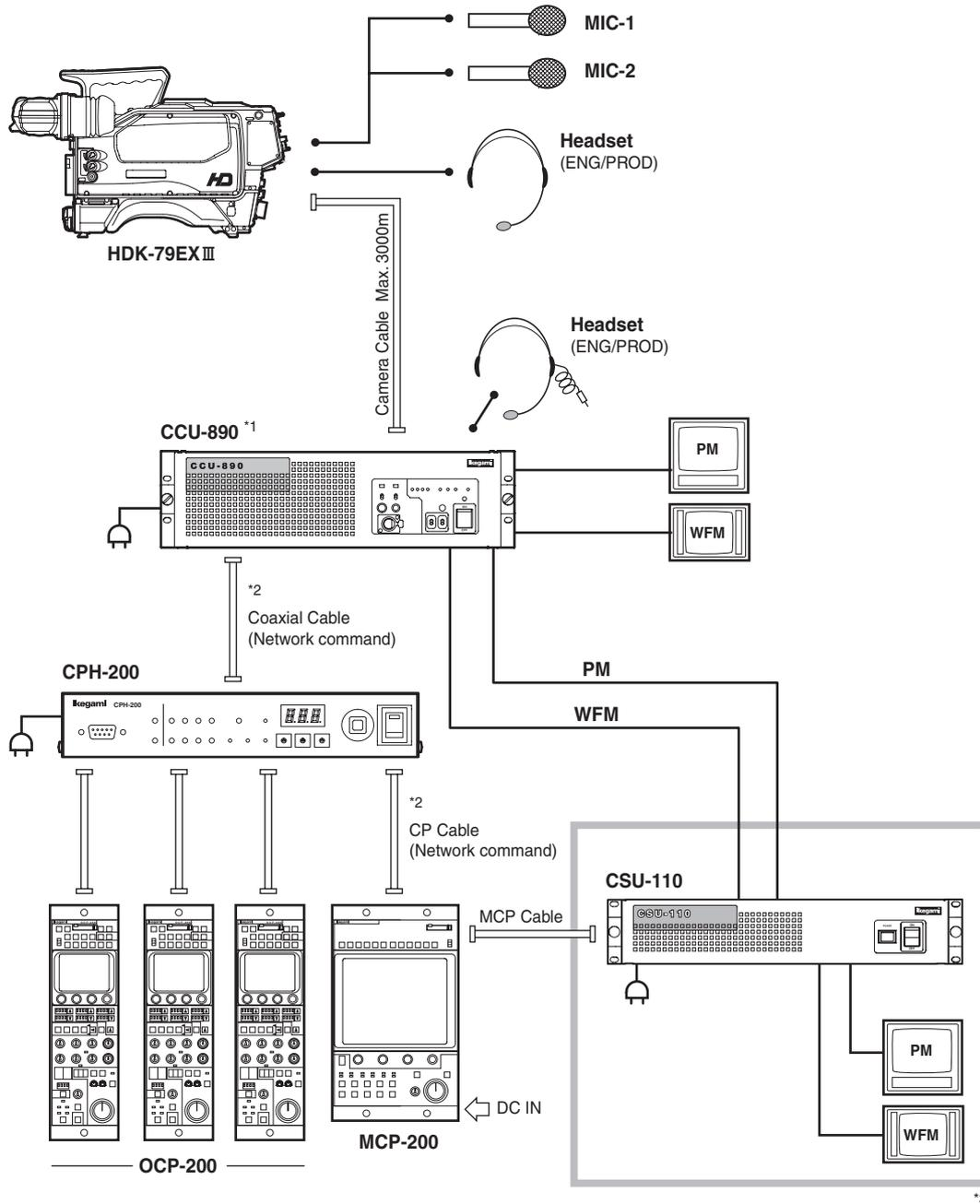
\*1 The CCU-890 can be operated when the network ID of the rotary switch on the PULSE module on the front of the CCU corresponds to the CCU No. set by an OPC or MCP.
