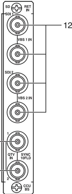
\* When the SD RET IN module is installed to this product, the QTV IN (QTV signal input) function is disabled for this connector.
