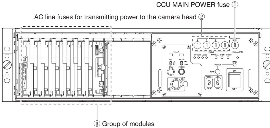
\* When the utility power output (UTILITY connector) on the camera head (studio camera) is not used, the CCU may not use AC line fuses No.3 and No.4 for transmitting power to the camera head.
