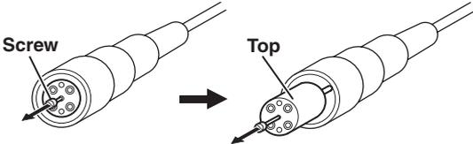
2 Pull the screw to remove the top from the connector.
