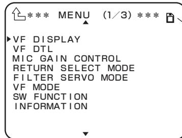
If the camera is recognizing the memory card normally, the memory card mark is displayed in the upper right of the VF menu screen.
