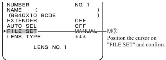
**M4** Turn the rotary pulse switch to switch the cursor on "MANUAL" to "OFF", and press the SET button to complete the lens file creation. Then, go to Step 8.
