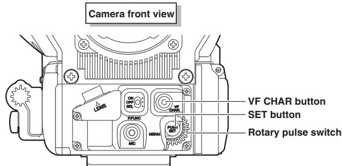
**Rotary pulse switch** : Used to select a setting item.
