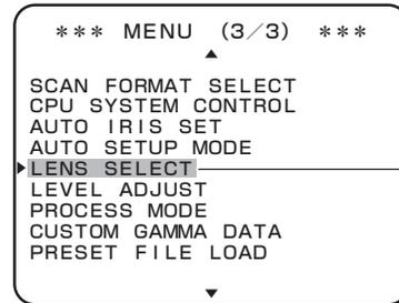
③ Position the flashing cursor on "LENS SELECT" and confirm.
