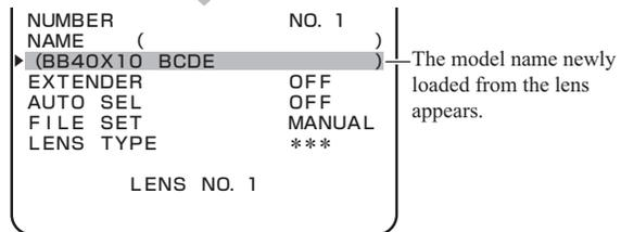
**M3** Turn the rotary pulse switch to position the cursor on "FILE SET", and press the SET button.
