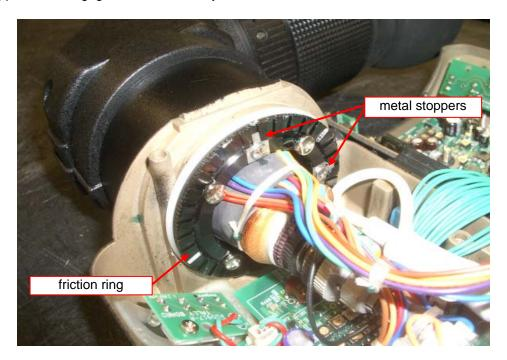
3) Tighten down stopper screws. Close the two half's of the viewfinder body.
