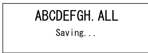
At the completion, the indication will come up on LCD screen and buzzer will beep. The indication will disappear 1.5 sec later.
