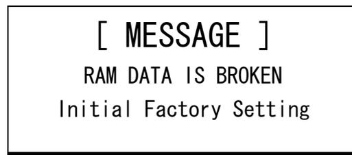
In this case, it is necessary to execute “18.3 Initial Factory setting” to reset to default factory setting.
