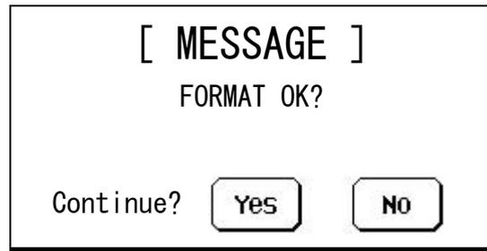
6. If [Yes] switch is pushed, card name will be changed immediately at the card name change, or format will be done immediately at the formatting. Buzzer will beep after execution is completed. Press [No] Switch it stop formatting.
