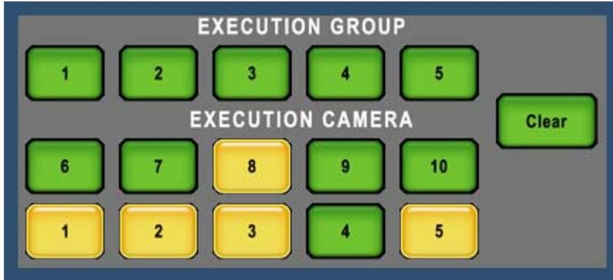
5. When the camera is selected in each group, and 50 cameras or less are executed at the same time, the group that is the setup is selected with the switch of EXECUTION GROUP. And the color of switch turns to amber. Selection will be cancelled by press the switch again.
