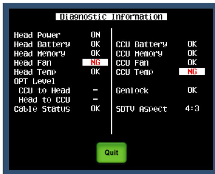
**CAUTION** With some type of BS/CCU, simple Diagnostic page on OCP may not be displayed, even though Diagnostic information is displayed on PM (Picture Monitor). This is not trouble but OCP could not get Diagnostic information from BS/CCU, because previous BS/CCU doesn't support this function.
