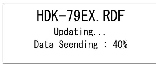
At the completing update, Complete Message window comes up and buzzer beep. Message window and buzzer will stop 1.5 sec. later.
