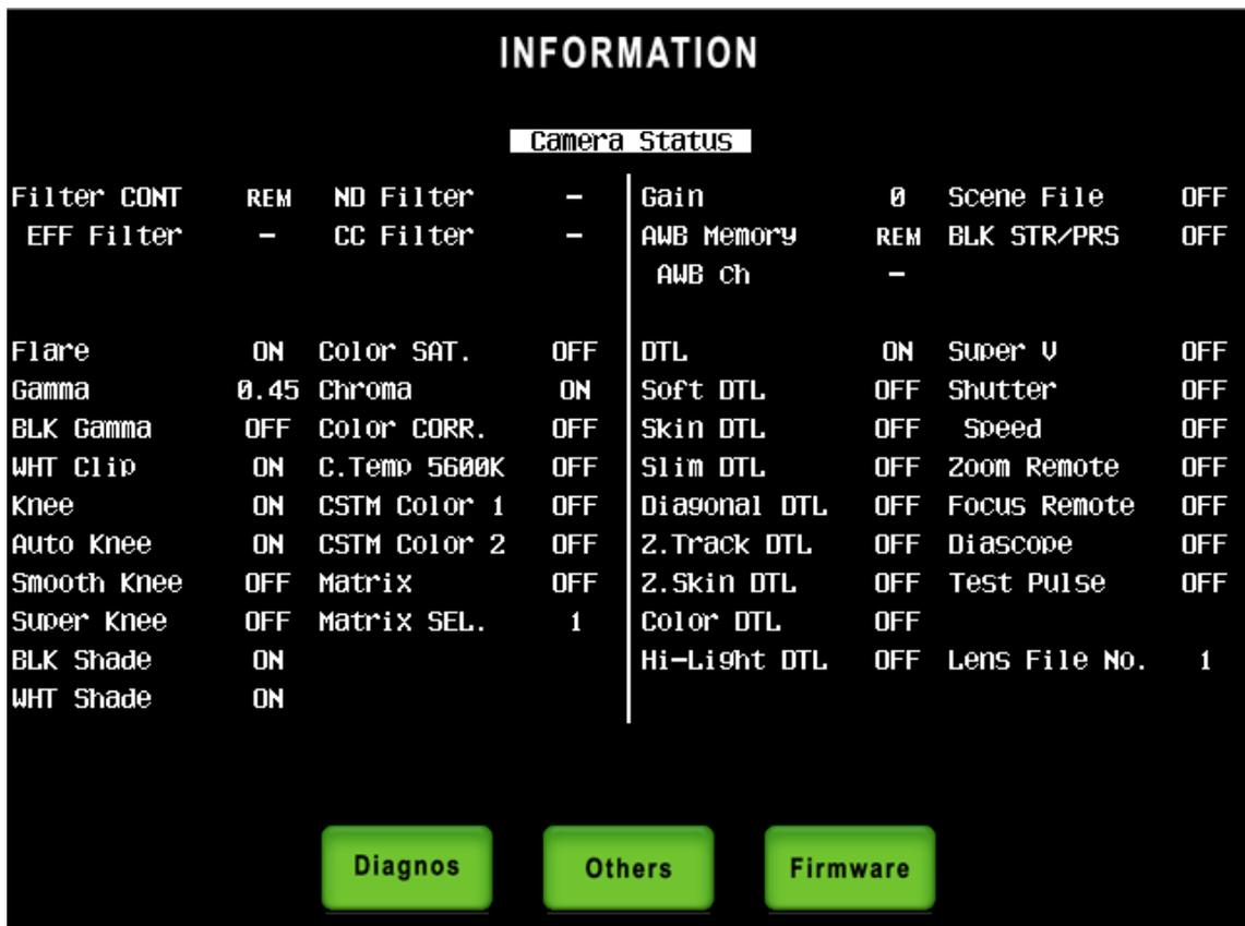
**CAUTION** Camera Status display page doesn't show all of camera function. Camera Control Function on top side and some of Select Switch Functions on middle of the panel of the panel and such as BARS ON/OFF and GAIN UP etc.
