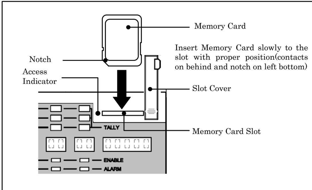
Note Do not extract Memory Card when access indicator on the slot lights or Saving/Loading data to/from Memory Card. Data or Card itself may be damaged.
