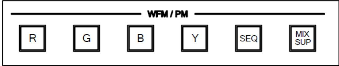
“R”, “G”, “B”, and “Y” can be output to the WFM output and the PM output. When “SEQ” is selected, three wave forms (R, G, and B) are output only as for the WFM output. To display treble signal on Waveform Monitor, it is necessary to connect WFM Remote Connector of BS/CCU to Waveform Monitor.
