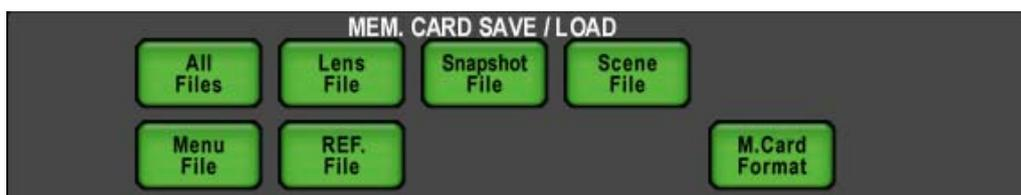
3. Select and push the switch for the type of data to be saved.
