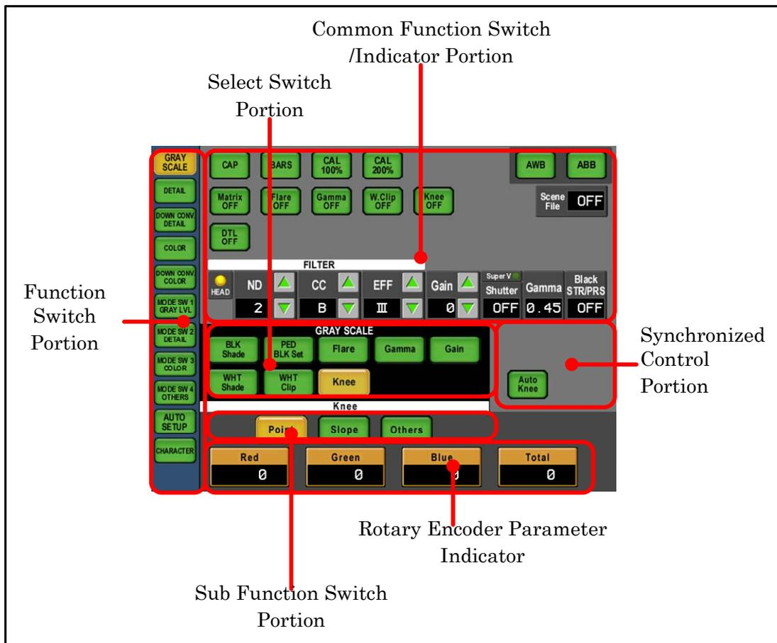
Switch icon on LCD and Rotary Encoder function display is classified by color. The color will change automatically by functionality of connected camera and BS/CCU.
