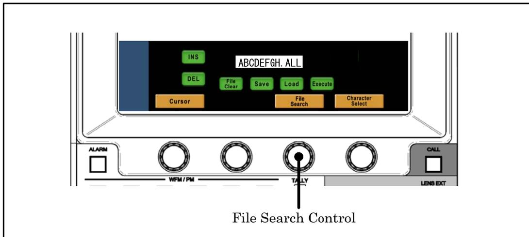
Note Push Name of File Data to indicate information of File Data to recognize sort of data file. And if CONTROL/SELECT Knob is rotated, following data will be indicated continuously.
