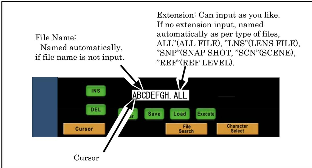
4. Input File Name by using switches on LCD and rotary encoder.
