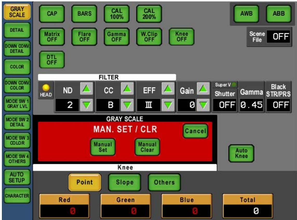
Turn the parameter to red, MANUAL SET / MANUAL CLR page will be overlaid. Click each of parameter to be done with MANUAL SET or MANUAL CLR. To identify the selection with turning parameter to red. To push the parameter(red number) again to release the setting.
