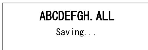
At the completion, the indication will come up on LCD screen and buzzer will beep. The indication will disappear 1.5 sec later.
