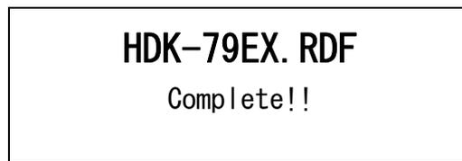
Confirm completion of firmware updating with VF, PM or Indicators of objective equipment. Set menu or switches back to previous setting.
