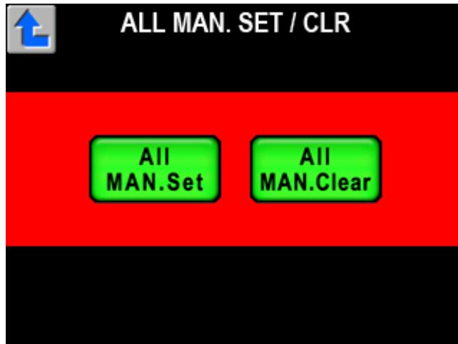
**Note** This operation executes Manual Set or Manual Clear for all control items, if control item is set OFF. However, some of functionality in Camera Head and BS/CCU doesn't apply to Manual Set and Manual Clear because of its specification.
