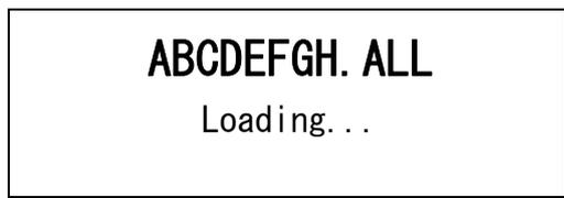
At the completion, the indication will come up on LCD screen and buzzer will beep. The indication will disappear 1.5 sec later.
