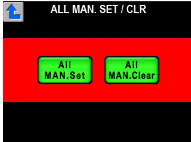
4. Press “ALL MAN. Set” for All Manual Set function or “ALL MAN. Clear” for All Manual Clear function. Switch will blink at the execution. And keep pressing until buzzer will beep.
