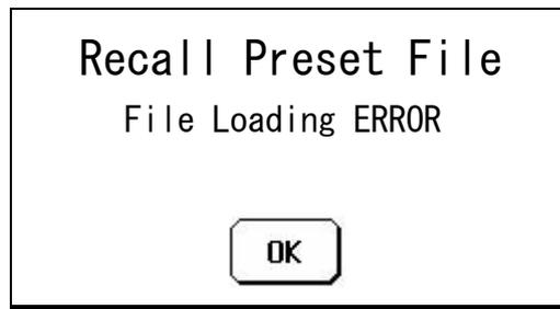
**Note** After Preset File loading, Camera Head and/or BS/CCU may be reset automatically for initialize. In that processing, OCP may be Panel Enable off or LCD screen off, but OCP is NOT in trouble. This is correct reaction because of unlocked command.
