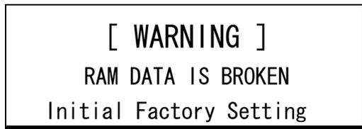
In this case, it is necessary to execute “13.3 Initial Factory setting” to reset to default factory setting.
