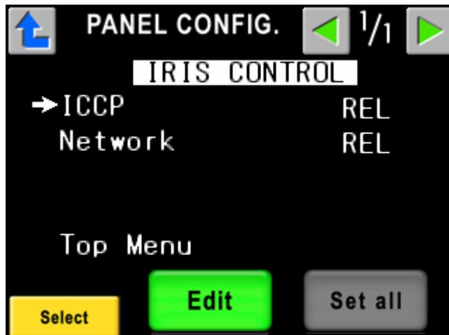
5. Selecting control item by Rotary Encoder, and press “Edit” switch. The entered setting is not final entry but it still temporary at this stage. If one of setting is changed, “Set all” will blink to indicate the change.
