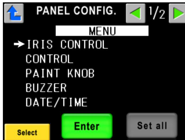
3. By rotating Rotary Encoder on left side, "→" symbol moves up and down. Set control item and push "Enter". Menu page can be changed with
