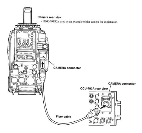
1 Connect the CAMERA connector on the rear of the CCU-790A to the CAMERA connector on the rear of the camera via a fiber cable.
