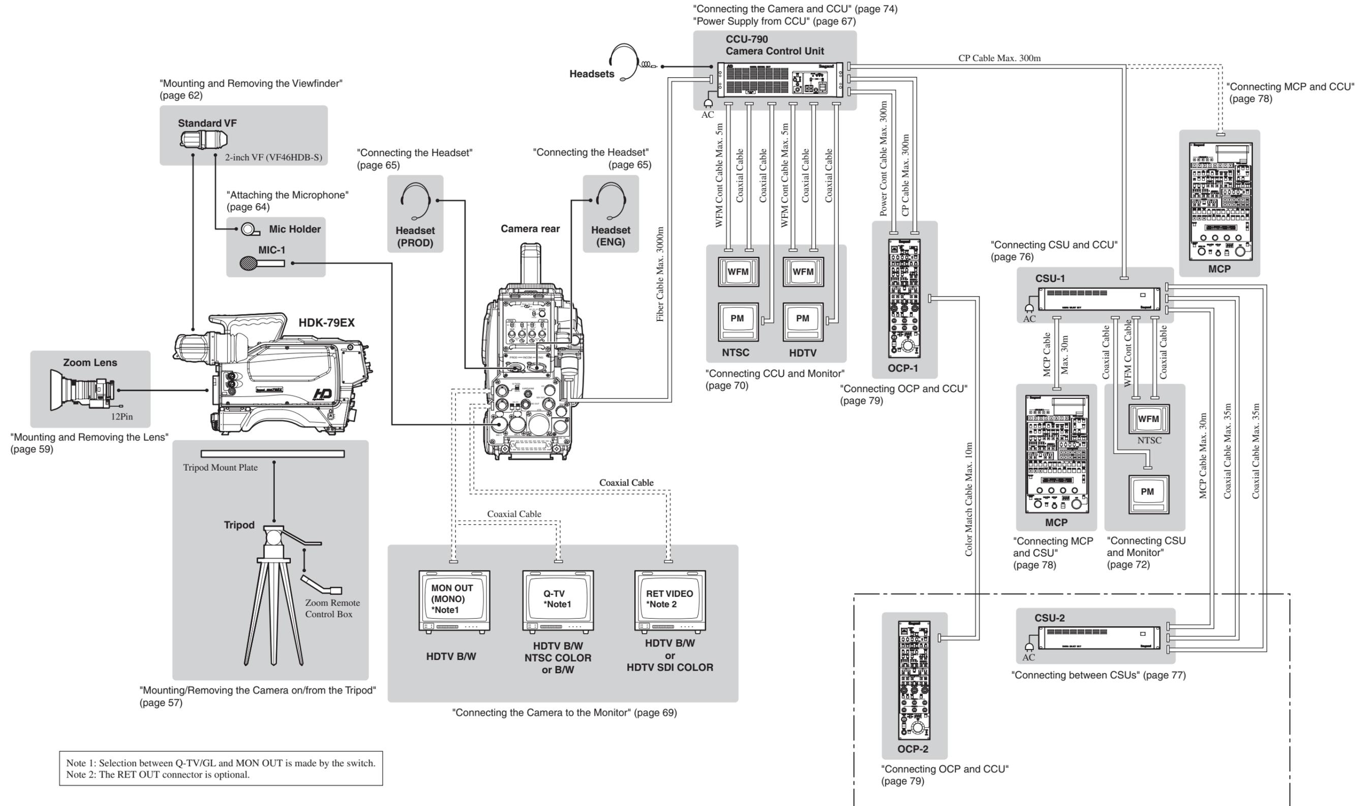
■ Connection Example for Studio Operation (Using CCU-790A)
