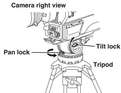
⑦ Loosen the tilt lock and pan lock and adjust the pan and tilt of the camera.
