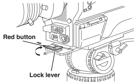
⑤ Tighten the lock lever until the camera is completely fixed.
