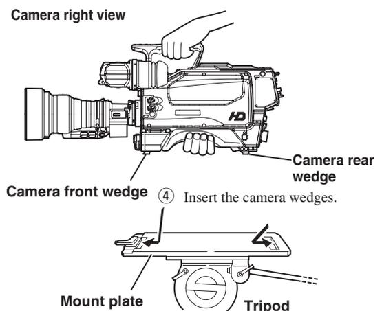
**5** After inserting the front wedge of the camera, tighten the lock lever until the camera is completely fixed.
