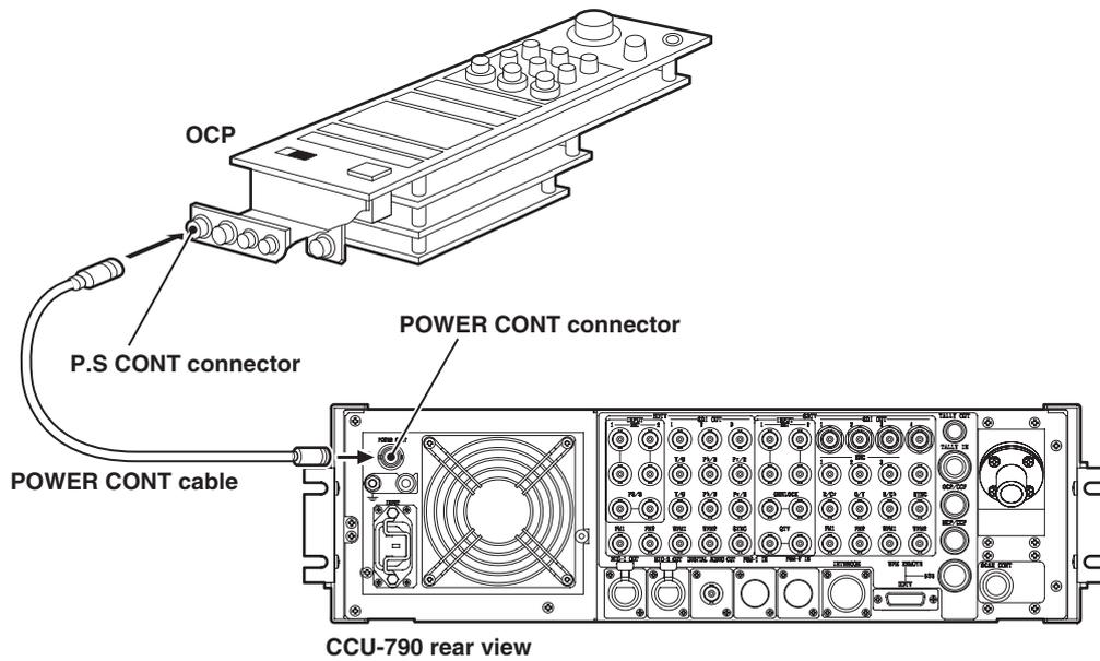
**5** Connect the POWER CONT connector on the rear of CCU-790 and the P.S CONT connector on the OCP via the POWER CONT cable.
