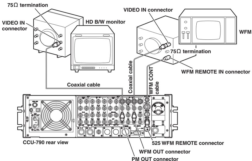
■ Connecting CCU-790A and Monitor
