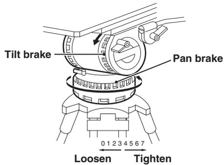
⑧ Tighten the tilt lock and pan lock to lock the camera.
