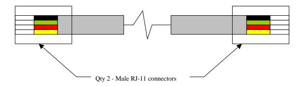
An RDU-1500 series UMD cable uses the center four pins of the RJ-11 connection. Connections are pin-to-pin, <u>unlike</u> the standard telco RJ11 cable, which uses a crossover connection.
