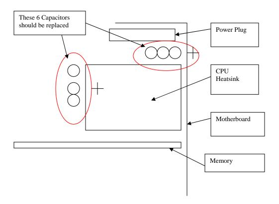
**Note**: Stripe on Capacitor marks negative side. Positive side is marked on motherboard at each capacitor position.
