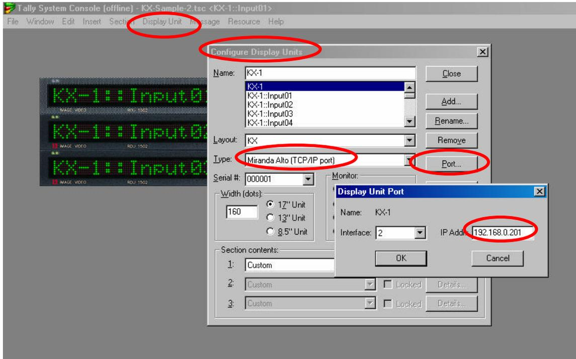
The Configure Display dialog is where the UMDs get set up. The “Name” list contains all of the UMDs. For each IP address there one display of “Type” - “Miranda Alto (TCP/IP port).” Clicking on that display in the name list and clicking on Port will take you to the sub-dialog where you can set the KX IP address. For each IP address (i.e. for each KX frame) you will have one of these “Miranda Alto (TCP/IP port)” displays.
