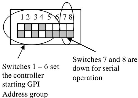
If there is only one TXI-series GPI controller connected to the tally controller, or if each TXI is connected to its own dedicated serial port and not daisy-chained to any other TXI, then all DIP switches 1-6 on each GPI controller can be set to the down position.
