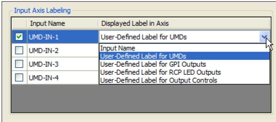
The input labeling style for more than one input item can be applied altogether. This is done by first selecting one or more input items. Afterwards, right-click the selection and choose Set Label for Selected Inputs. Select which labeling style to apply.
