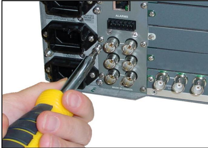
**Figure 4-6.** Re-installing the Mounting Screw
