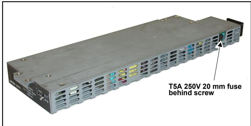
**Figure 4-8.** Location of Fuse in 3901PS Power Supply Module
