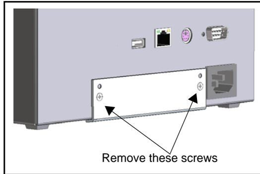
**Figure 1-6.** Removing the Stabilizer Bracket
