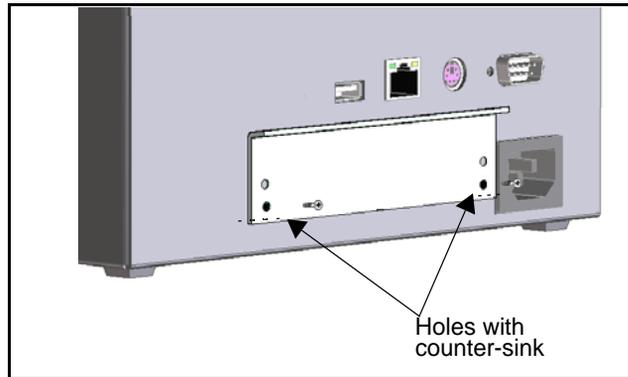
**Figure 1-8.** Attaching the Stabilizer Bracket to NUCLEUS-DM
