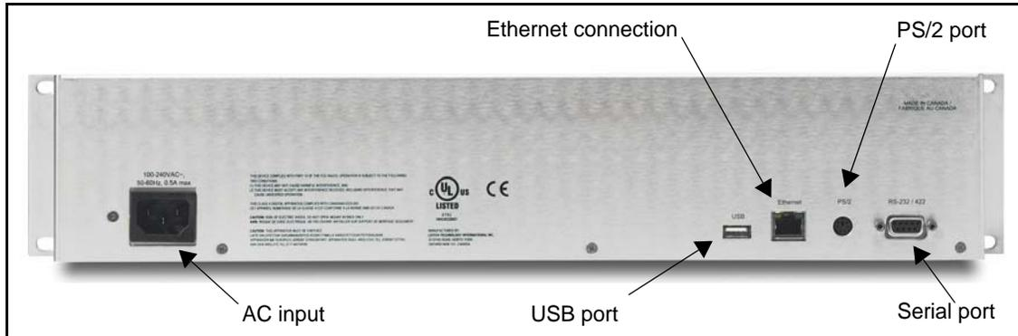
Figure 1-3. Back View of NUCLEUS Rack-Mount Control Panel
