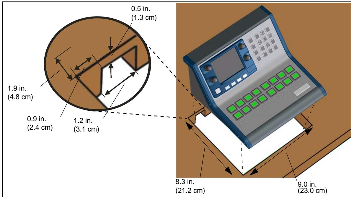
**Figure 1-9.** Mounting NUCLEUS-DM into the Cutout
