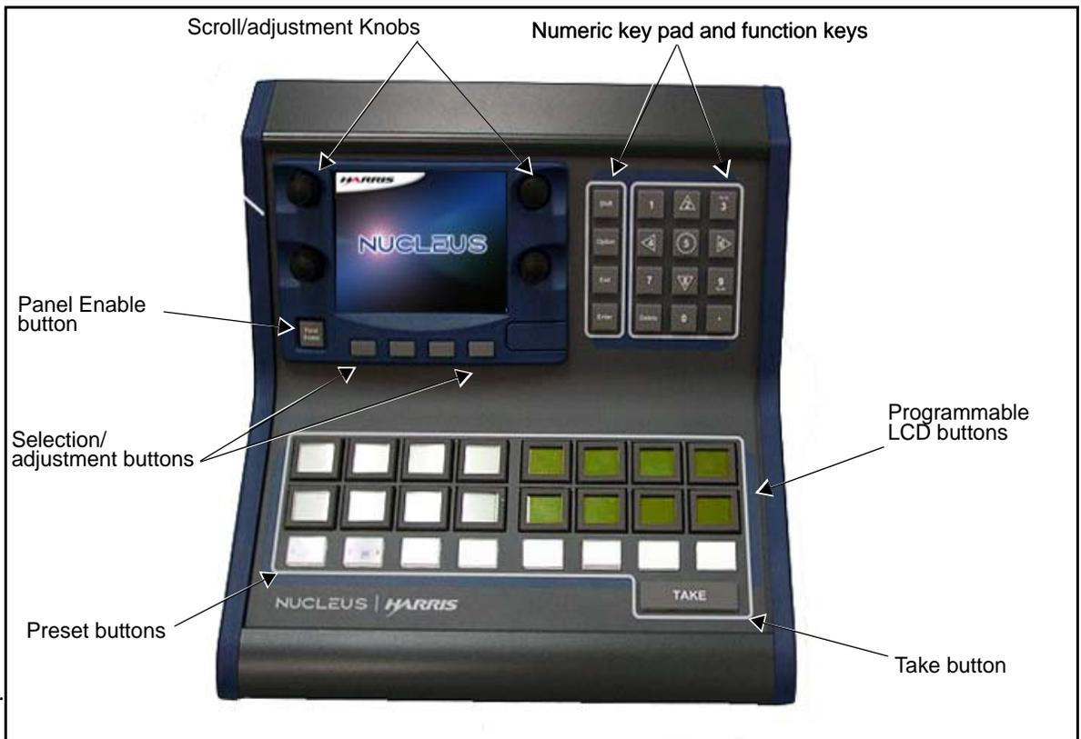
**Figure 1-2.** Front View of NUCLEUS-DM Desk-Mount Control Panel
