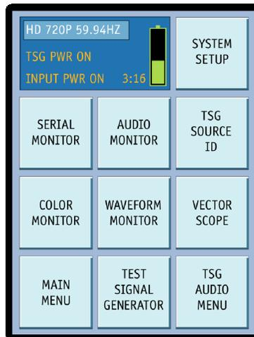
The HD-STAR main menu is the first screen to appear after the unit is powered on. The **MAIN MENU** button is always active in the lower-left corner of the screen, even though it is not seen on some screens. To return to the main menu just tap the stylus on the lower left of any screen.
