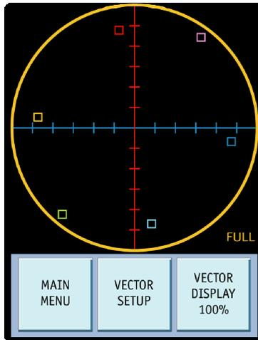
The Vector Scope screen is used to measure the vector of the SD or HD input. The vector display itself is a yellow circle with a blue horizontal graticule and red vertical graticule. The color boxes in the vector display represent the actual colors being measured: Green, Yellow, Red, Magenta, Blue, and Cyan.
