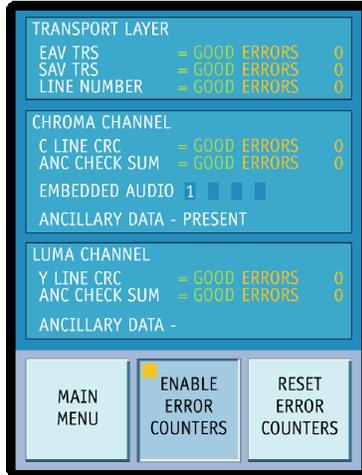
The Serial Monitor screen is used to measure the number and type of errors that occur on the serial input. If everything is acceptable for a particular measurement, GOOD is displayed on the line. During an error, the GOOD indication changes to BAD and the number of times the error occurs is counted. The errors are measured on the following parameters:
