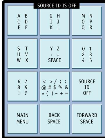
The TSG SOURCE ID menu is used to control the internal character generator. The character generator can insert text into the output of the test signal generator. There are five 18-character identifier outputs through both outputs.
