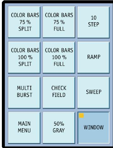
The HD-STAR outputs an HD signal when HD mode is selected in the SYSTEM SETUP menu. The Test Signal Generator screen is used to set up the HD test signal for the output. The selections are:
