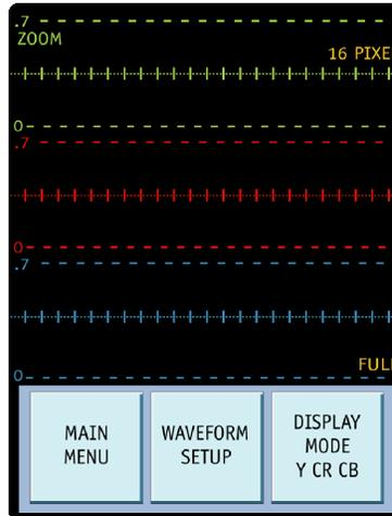
The Waveform Monitor screen shows the 1H waveform of the input video. Two display modes are available with the DISPLAY MODE button in the waveform display: YC<sub>R</sub>C<sub>B</sub> and GRB. YC<sub>R</sub>C<sub>B</sub> mode displays the waveform in a luma, component blue, and component red representation. GRB displays the waveform into a green/red/blue component representation.
