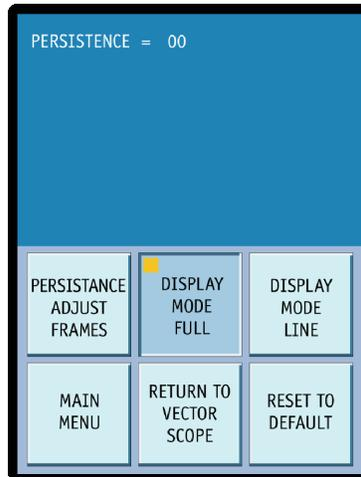
The VECTOR SETUP menu contains the RESET TO DEFAULT selection. Pressing the RESET TO DEFAULT buttons sets the Persistence to 80, and the Display Mode to FULL.
