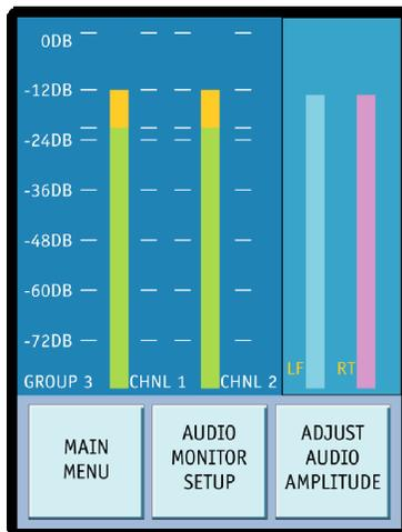
The audio monitor screen displays two channels of audio. The channels that appear on the display are determined by the selection made in the AUDIO MONTOR SETUP menu.
