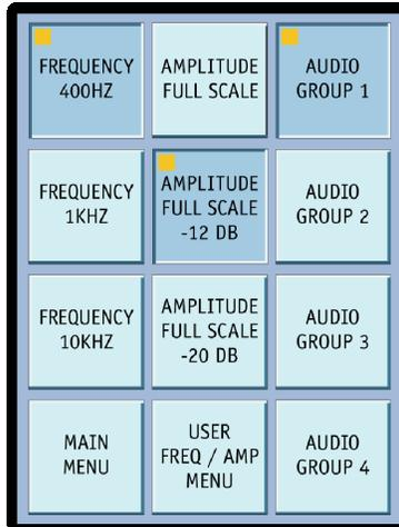
The TSG (Test Signal Generator) AUDIO MENU is used to select the embedded audio for the SDI test signal generator output.
