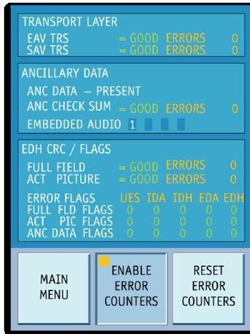
The Serial Monitor screen is used to measure the number and type of errors that occur on the serial input. If everything is acceptable for a particular measurement, GOOD is displayed on the line. During an error, the GOOD indication changes to BAD and the number of times the error occurs is counted. The errors are measured on the following parameters:
