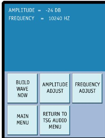
The USER FREQ/AMP MENU button in the TSG Audio Menu screen is used to access the User Freq/Amp Menu screen. Once the screen is accessed, press the AMPLITUDE ADJUST or FREQUENCY ADJUST button. Move the stylus up and down in the blue area of the screen to adjust the Amplitude or Frequency values. The changes occur when the BUILD WAVE NOW button is selected. The RETURN TO TSG AUDIO MENU button is used to return the display to the TSG AUDIO MENU screen.
