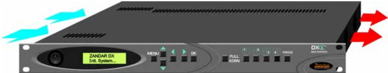
Figure 3: MultiViewer airflow diagram
