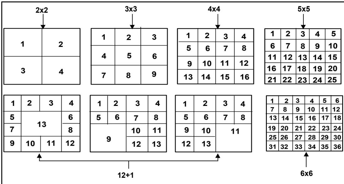
**Figure 3-1.** Preset Display Layouts
