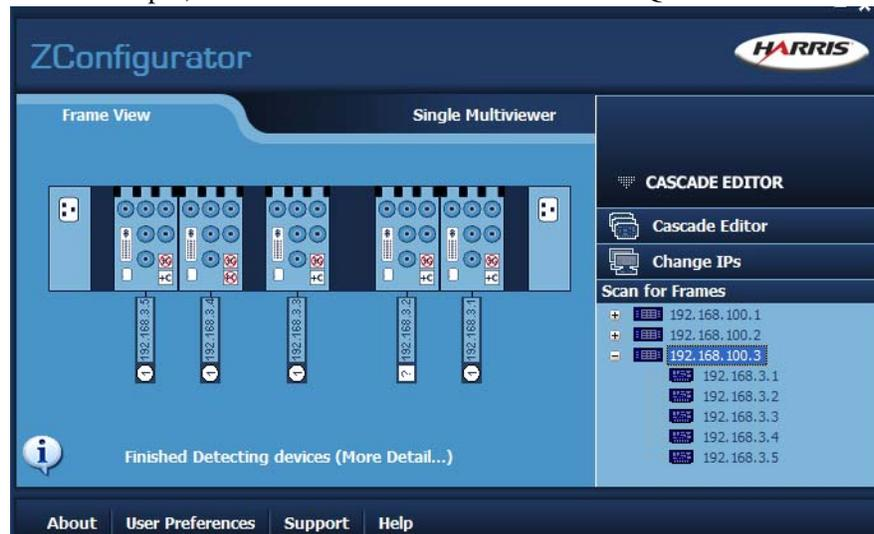
There are four standalone quad cards, (shown with white circles with a '1' in them) in the frame with IP 192.168.100.3. One quad card is shown with a question mark '?' in a white square. This indicates that it is a slave card that has become orphaned and is no longer associated with a master card. This card can be made available for the new cascade from within the editor using the **Break** command as we will see later.
