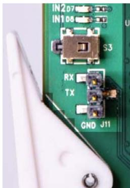
**Figure 7-6.** Serial Port on Card Edge
