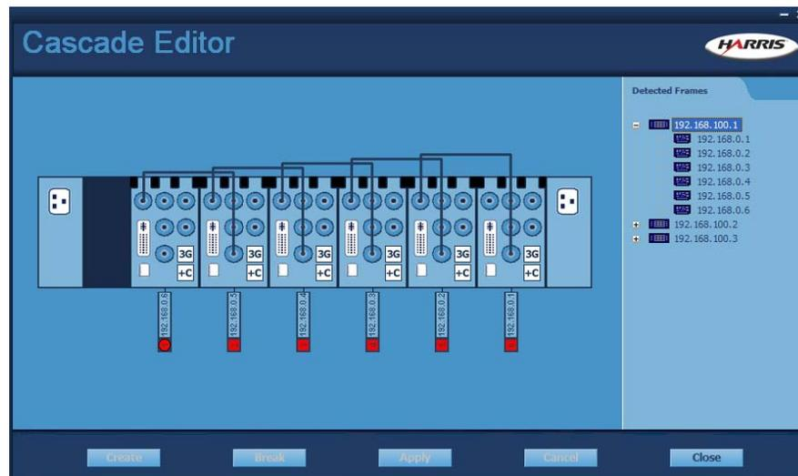
In the above example, a virtual multiviewer with 24 inputs has been created out of six QVM6800+C-T cards from one frame.
