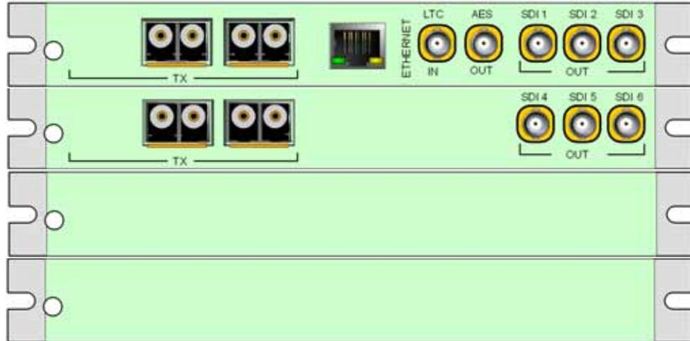
**Figure 1-10** HV-SXP-64x6-O or HV-SXP-32x6-O-FR28 Back Module
