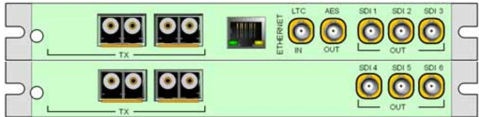
**Figure 1-8** HV-SXP-32x6-O or HV-SXP-16x6-O-FR28 Back Module
