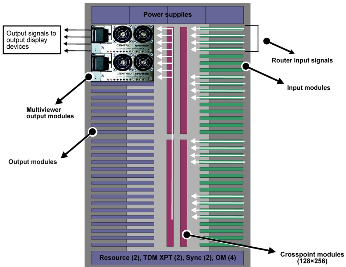
**Figure 3-1.** Platinum 15RU Router Frame with Output Modules
