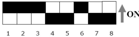
**Figure 3-6.** eBOX Dip Switch Settings for Operation
