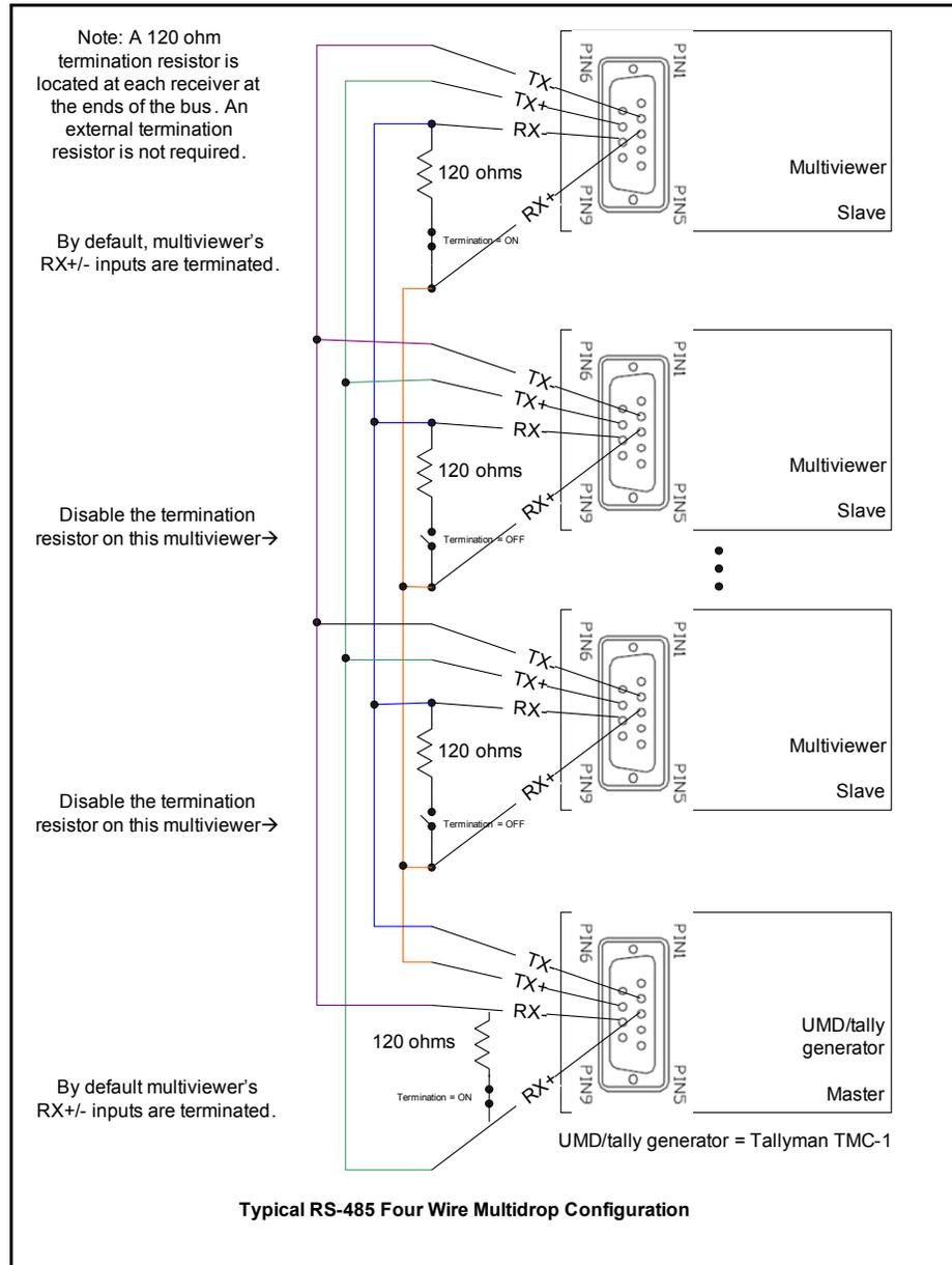
Figure C-1. Typical RS-485 Four Wire Multidrop Configuration
