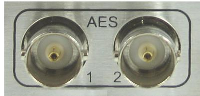
Standard coaxial/unbalanced output audio connectors
