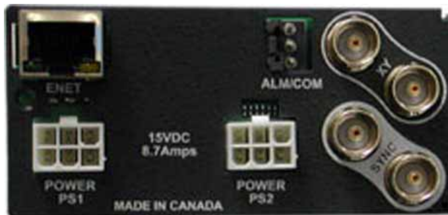
Figure 1-10 X-Y/Genlock Connector Orientation
