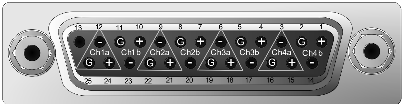
Figure 1-4 Female Back Panel Analog Audio Input and Output Pinouts
