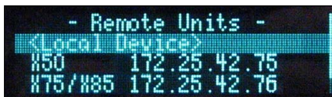
Figure 2-11. List of Systems Available for Remote Control
