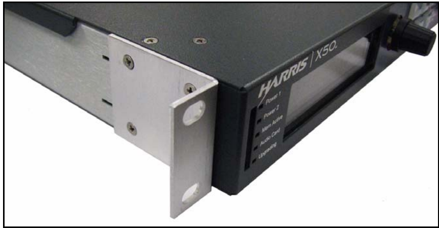
Figure 2-1. Mounting Ears in Front Position
