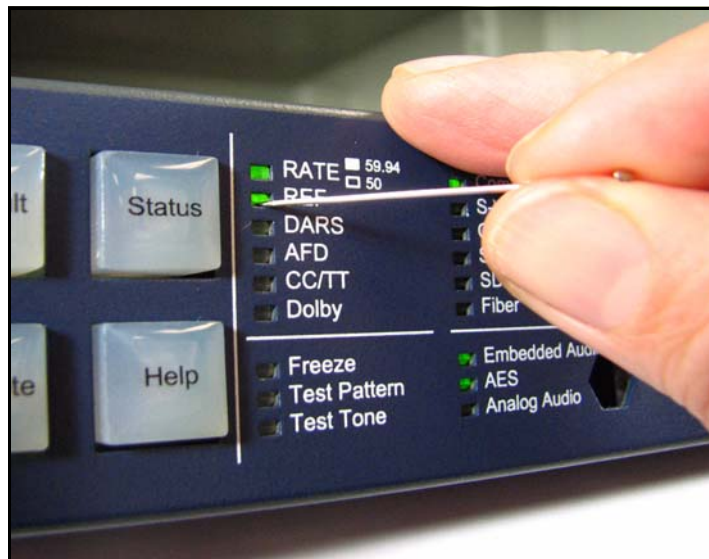
Figure 2-7. Re-Aligning Rubberized Light Tubes
