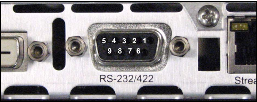
Figure C-41. Data Port Pinouts
