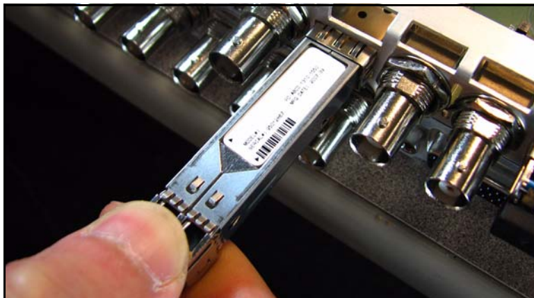
Figure C-22. Inserting the SFP Module
