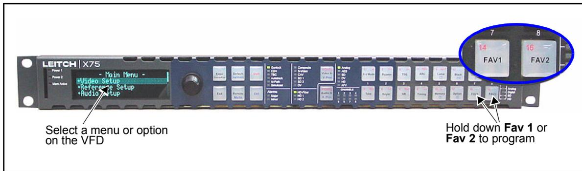
**Figure 2-13.** User-Programmable Controls
