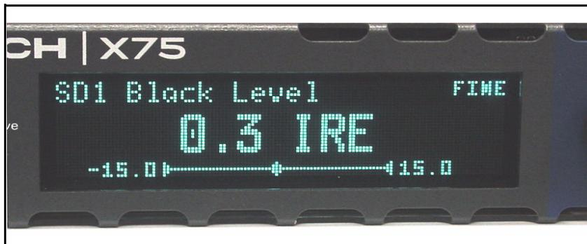
**Figure 2-3.** VFD Panel Showing Numerical Range of Values
