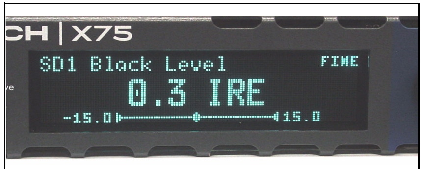
Figure 2-3. VFD Panel Showing Numeric Range of Values
