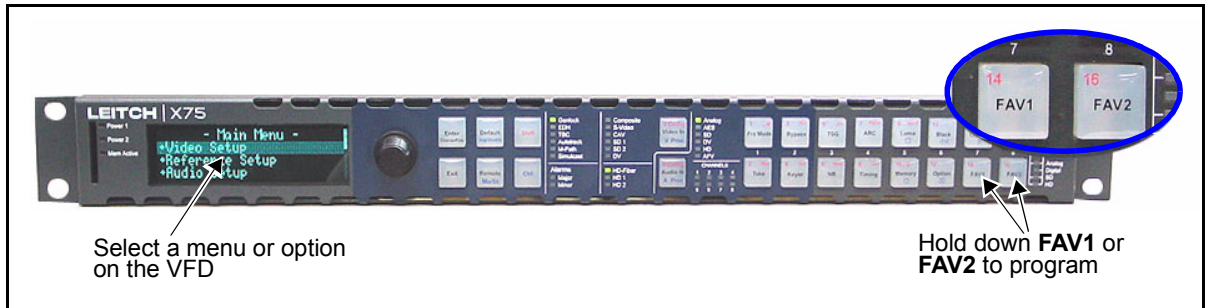
Figure 2-11. User-Programmable FAV1 and FAV2 Controls
