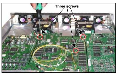
Figure C-38. Removing HDTV Board Mounting Screws
