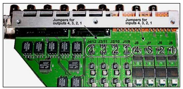
Figure 1-3. Jumper Locations for X75OPT-AS-16 and X75OPT-AS-8 Modules
