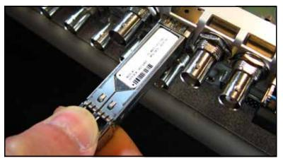
Figure C-22. Inserting the SFP Module
