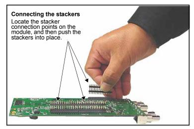
Figure C-24. Connecting Three Stackers to Module
