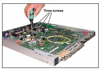
Figure C-37. Removing Audio Board Mounting Screws
