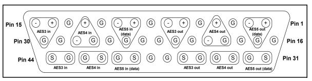
Figure A-12. CAB-X75HD-COMBO Connector Pinout
