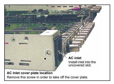
Figure C-50. Removing Cover Plate and Installing AC Inlet
