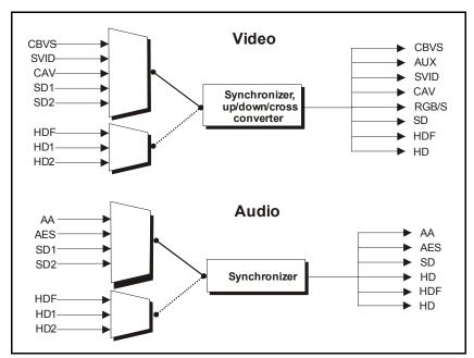
Figure 2-12. X75 Simulcast Processing
