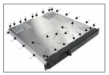
Figure C-34. Chassis Cover Screws
