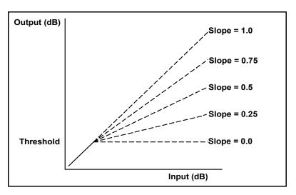
Figure 1-5. Audio Limiter Transfer Function
