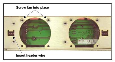
Figure C-56. Replacing a Fan within the Assembly
