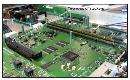
Figure C-16. Stackers on the Main Board
