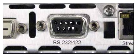
Figure C-41. Data Port Pinouts
