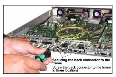
Figure C-15. Securing the Back Connector to the Frame
