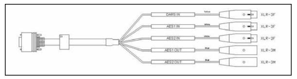
Figure A-13. X75OPTCAB-8-X Cable Connectors
