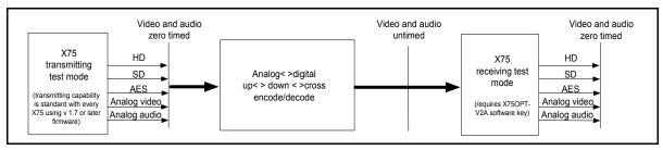
Figure 8-2. X75OPT-V2A Video/Audio Timing Feature
