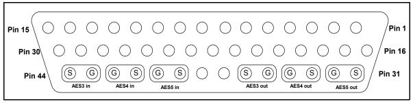
Figure A-8. CAB-X75HD-COAX Connector Pinout
