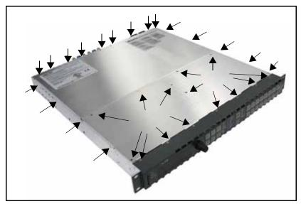
Figure C-2. Location of Chassis Cover Screws
