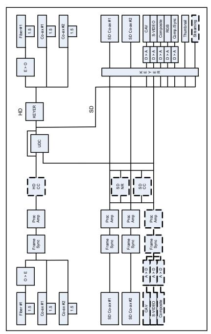
Figure 1-14. X75 Signal Flow
