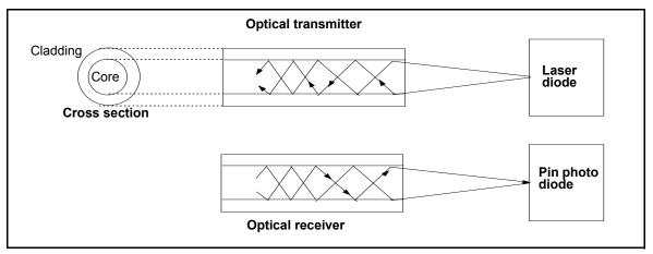
Figure C-1. Fiber Optic Transmitting and Receiving
