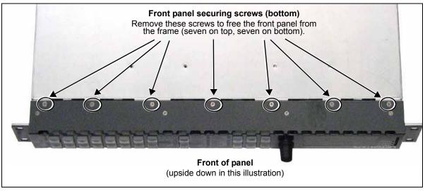
Figure C-53. Freeing the Front Panel from the Frame
