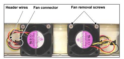
**Figure C-55.** Removing Header Wires from Fan Assembly Connector
