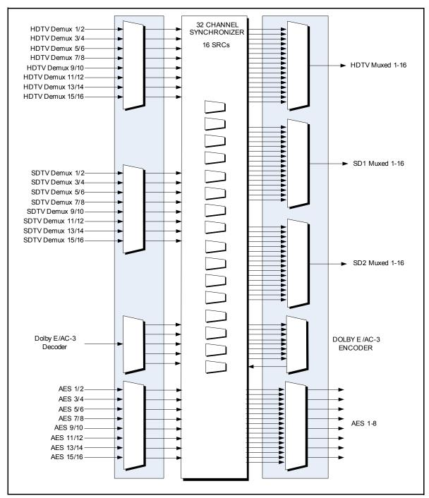
Figure 2-10. 32-Channel Audio Functional Block Diagram
