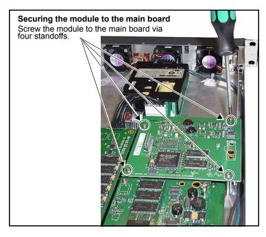
Figure C-30. Securing the Module to the Main Board
