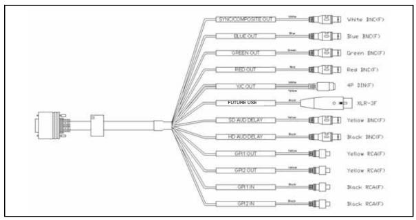
Figure A-2. X75OPTCAB-MULTI Cable Connectors
