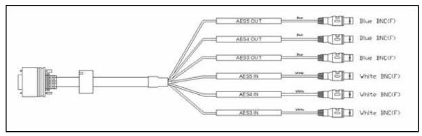
Figure A-7. CAB-X75HD-COAX Cable Connectors
