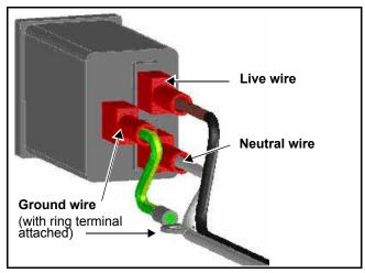
Figure C-51. Connecting AC Cables to Inlet
