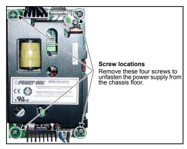
Figure C-45. Removing the Power Supply
