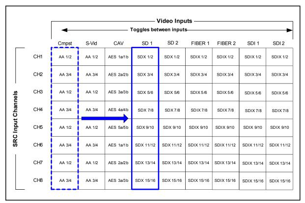
Figure 9-4. X85 Default AFV Channel Assignment
