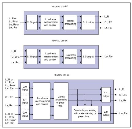
Figure 9-15. DTS Neural Audio Option Block Diagrams (3)
