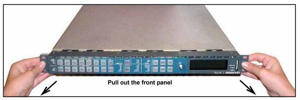
Figure C-54. Removing the Front Panel
