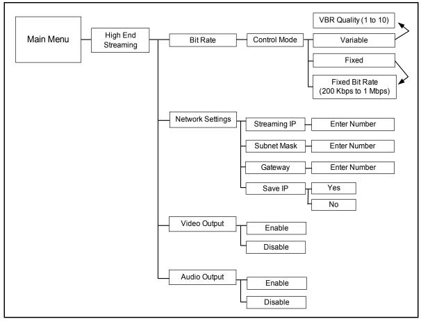
Figure C-31. Streaming Module Settings
