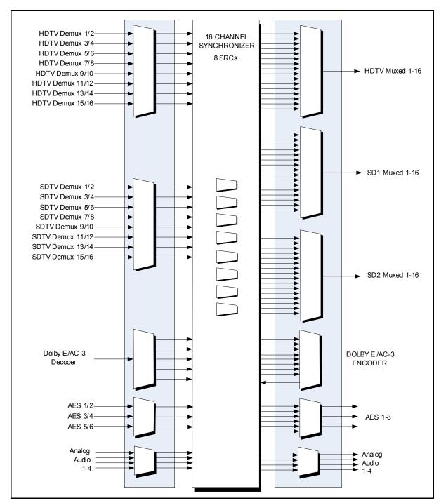
Figure 2-9. 16-Channel Audio Functional Block Diagram
