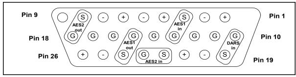
Figure A-6. X75OPTCAB-8-C Connector Pinout
