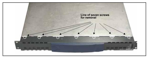
Figure C-3. Removing the Bottom Front Panel Screws
