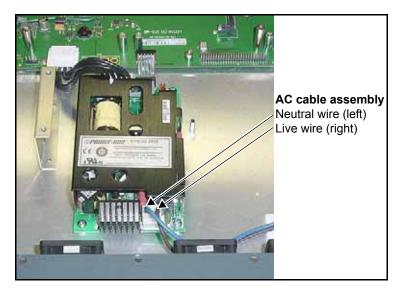
Figure C-48. Connecting AC Cables to Power Supply
