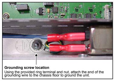
Figure C-52. Grounding AC Inlet
