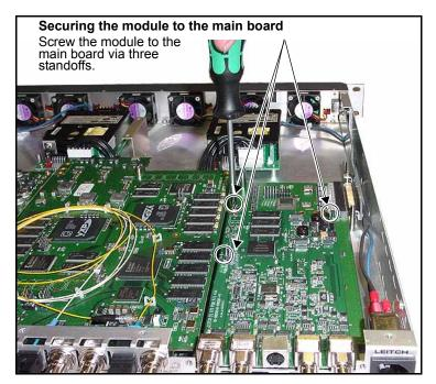
Figure C-28. Securing the Module to the Main Board
