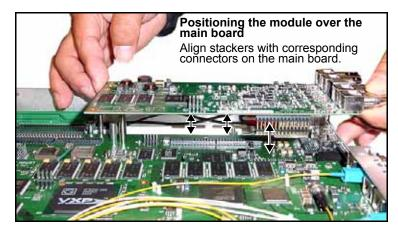
Figure C-26. Positioning Module over Standoffs
