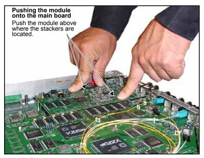
**Figure C-27.** Pushing the Module on to the Main Board (X75 Shown)
