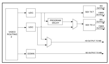
Figure 2-4. X85 Program Delay Mode
