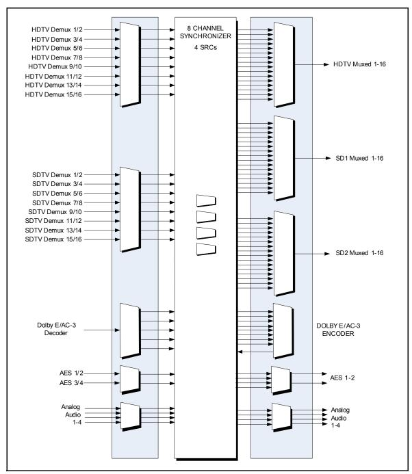
Figure 2-8. Eight-Channel Audio Functional Block Diagram
