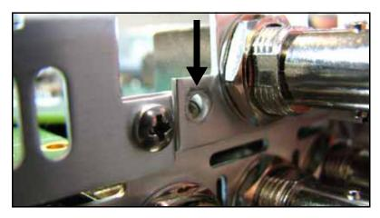
Figure C-19. Aligning the Back Panel
