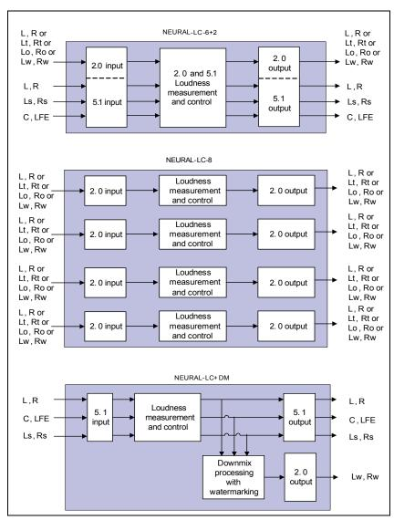
Figure 9-14. DTS Neural Audio Option Block Diagrams (2)
