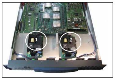
Figure C-46. Where to Install a Redundant Power Supply
