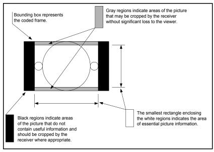
Figure 8-16. AFD Diagram Explanation
