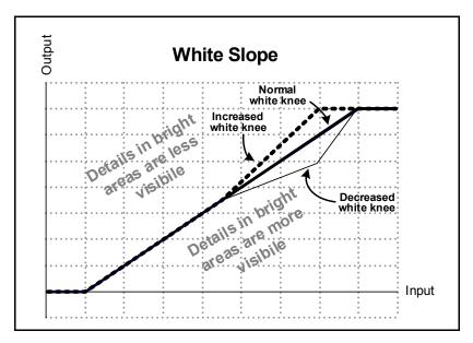
Figure 8-25. Examples of Increased and Decreased White Slope
