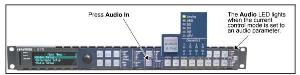
Figure 9-1. Audio Input Control Area (X75 Shown)
