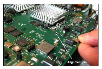
Figure C-18. Alignment Pin for the X85 Module
