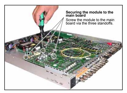
Figure C-8. Securing the Module to the Main Board
