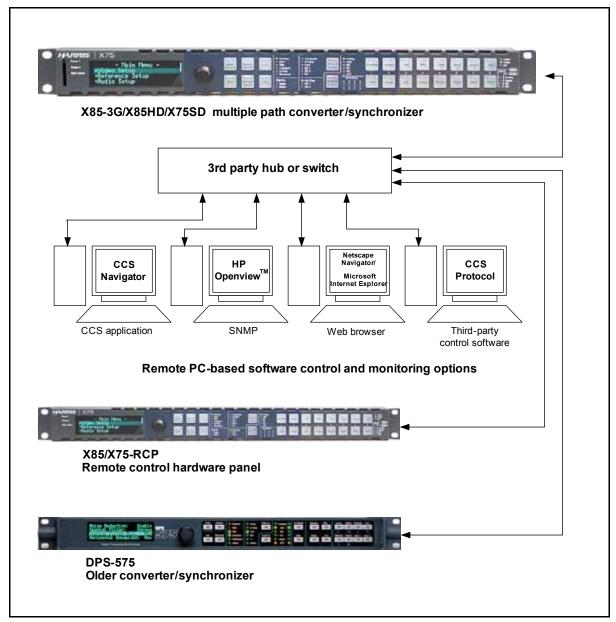
Figure 1-12. Typical Configuration, Control, and Monitoring Methods
