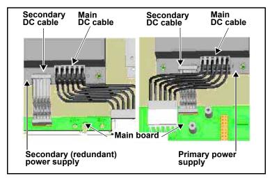
Figure C-47. Connecting DC and Ribbon Cables
