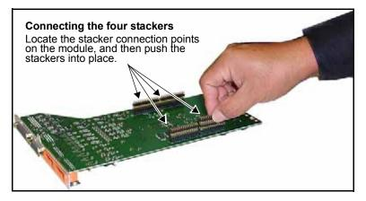
Figure C-4. Connecting Four Stackers to Module
