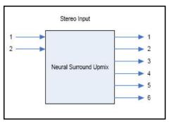
Figure 9-16. UpMix Block Diagram
