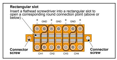
Figure 1-4. Installing Analog Audio Receptacles
