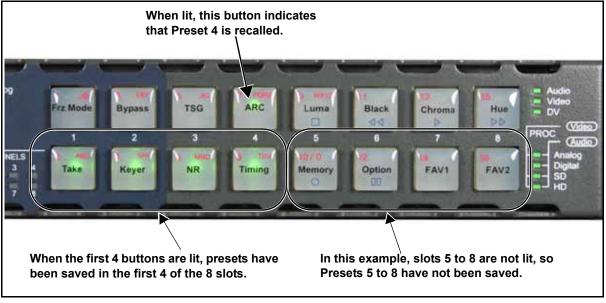
Figure 5-3. Example of Preset Slots Saved
