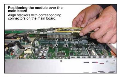
**Figure C-12.** Positioning Module over Standoffs
