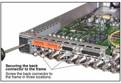
Figure C-9. Securing the Back Connector to the Frame
