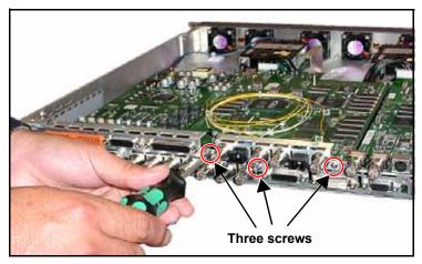
**Figure C-36.** Removing HDTV Back Module Screws (X75OPT-HDUPG HD Module Shown)
