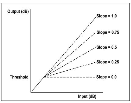
Figure C-32 shows the transfer function of the Audio Limiter:
