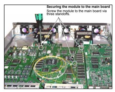
Figure C-14. Securing the Module to the Main Board
