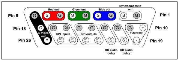
Figure A-3. X75OPTCAB-MULTI I/O Connector Pinout
