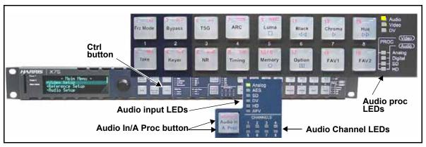
Figure 9-2. Location of Audio LEDs (X75 Shown)
