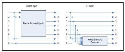
Figure 9-18. MultiMerge Block Diagram
