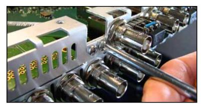
Figure C-21. Securing the Back Connector to the Frame
