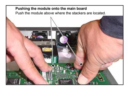
Figure C-29. Pushing the Module on to the Main Board
