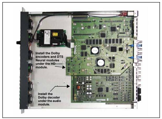
**Figure C-33.** Locations of Dolby and DTS Neural Modules (X75OPT-HDUPG HD Module Shown)
