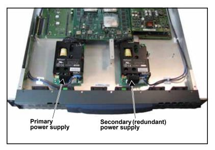
Figure C-42. Location of Connected Power Supply
