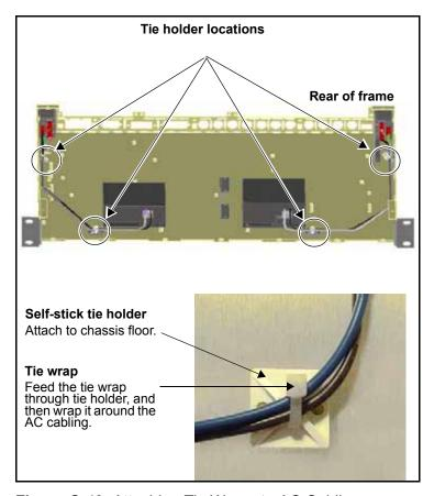
Figure C-49. Attaching Tie Wraps to AC Cabling
