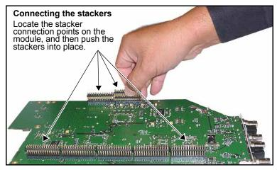
Figure C-10. Connecting Seven Stackers to Module
