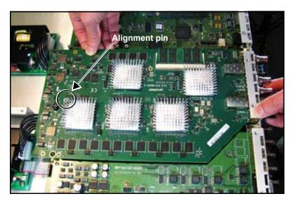
**Figure C-17.** Positioning the X85 Module
