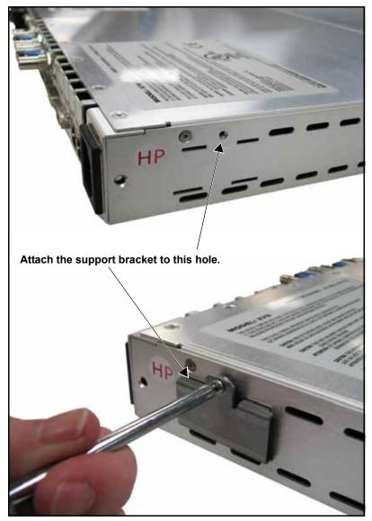
Figure 4-2. Bracket Installation
