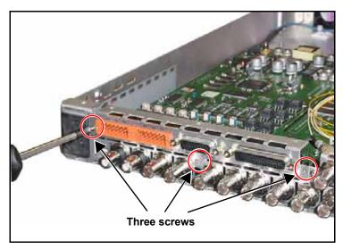
Figure C-35. Removing Audio Back Module Screws
