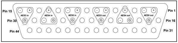
Figure A-16. X75OPTCAB-XLR Connector Pinout
