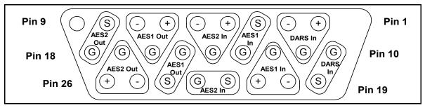
Figure A-10. X75OPTCAB-8-XC Connector Pinout
