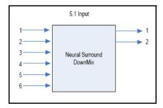
Figure 9-17. DownMix Block Diagram
