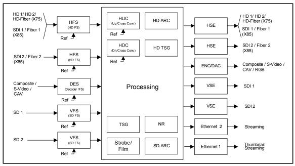
Figure 2-1. Video Functional Block Diagram
