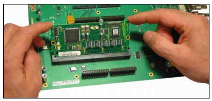
Figure C-39. Inserting Dolby Decoder Module into Socket
