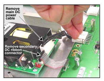
Figure C-43. Removing the DC and Ribbon Cables
