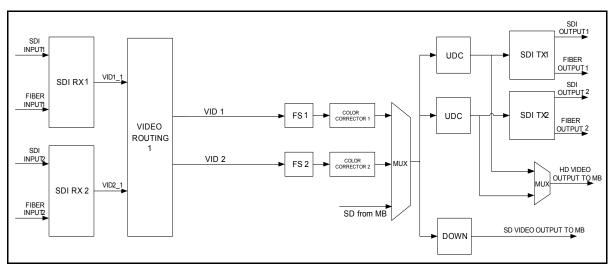
Figure 2-3. X85 Simulcast/All Output Select
