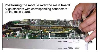
Figure C-6. Positioning Module over Standoffs
