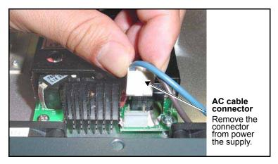
Figure C-44. Removing AC Cable from Power Supply
