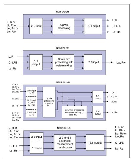
Figure 9-13. DTS Neural Audio Option Block Diagrams (1)
