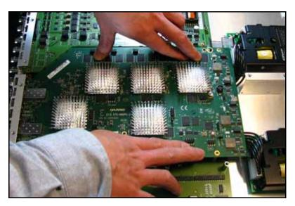
Figure C-20. Pushing the Module Onto the Main Board
