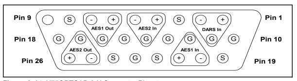
Figure A-14. X75OPTCAB-8-X Connector Pinout
