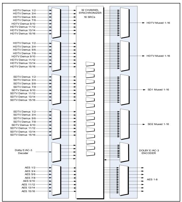
Figure 2-11. 32-Channel 3 Gb/s Audio Functional Block Diagram
