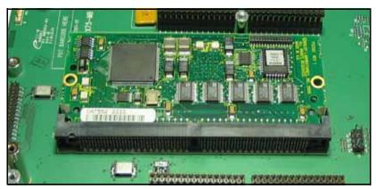
Figure C-40. Dolby Decoder Module Installed
