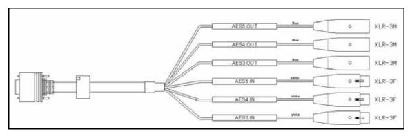
Figure A-15. X75OPTCAB-XLR Cable Connectors
