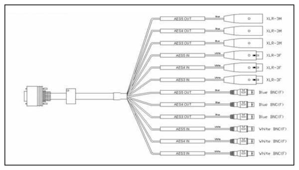
Figure A-11. CAB-X75HD-COMBO Cable Connectors
