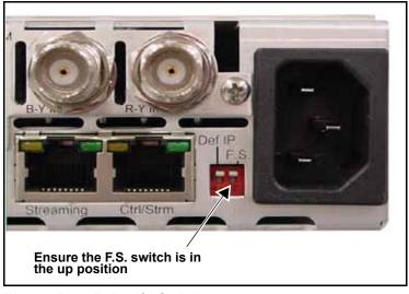
Figure B-2. Fail-safe Switch
