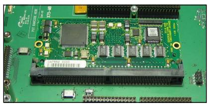
Figure C-40. Dolby Decoder Module Installed
