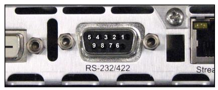
Figure C-41. Data Port Pinouts
