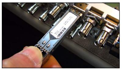
Figure C-22. Inserting the SFP Module
