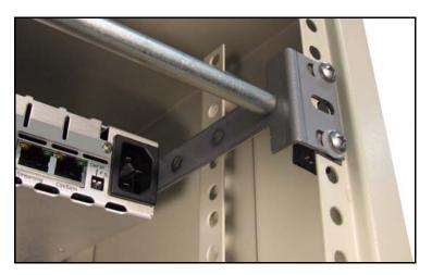
Figure 4-4. Installed Support Arms
