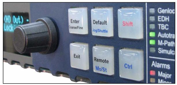
Figure 5-1. Control Knob and Menu Control Area
