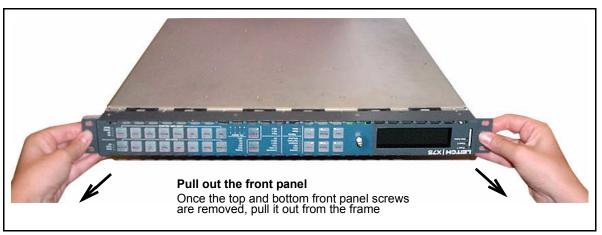
Figure C-34. Removing the Front Panel
