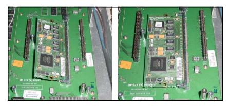
Figure C-22. Dolby Decoder Module Installation
