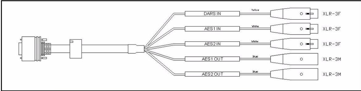
Figure A-13. X75OPTCAB-8-X Cable Connectors
