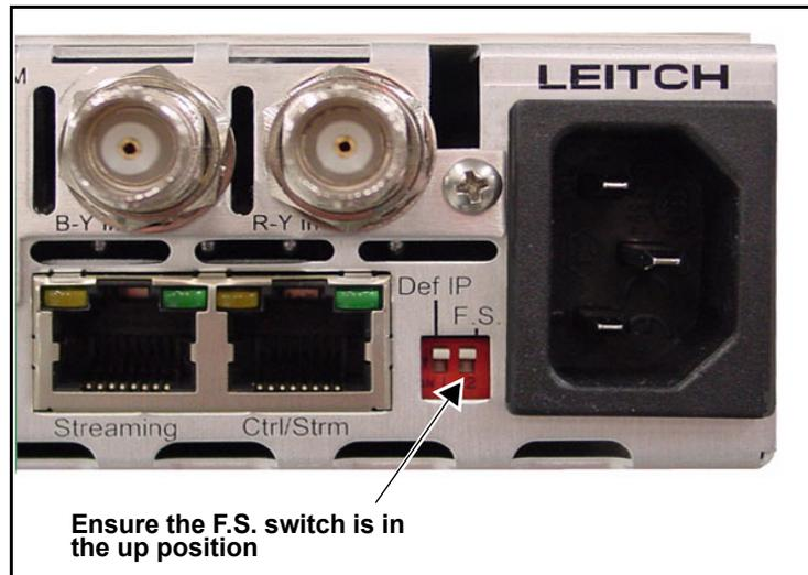
**Figure B-2.** Fail-safe Switch
