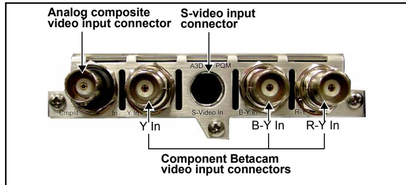
**Figure 3-5.** X75OPT-A3D Module Back Panel
