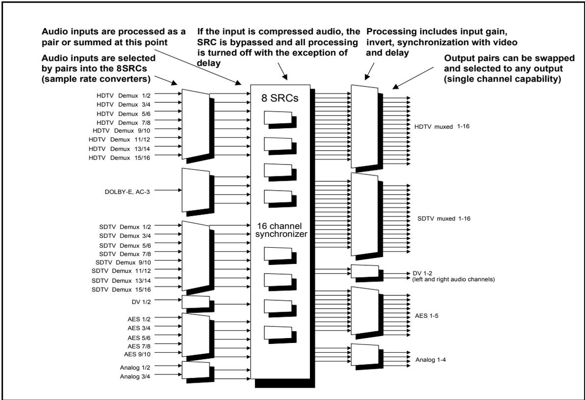
**Figure 1-8.** Audio Functional Block Diagram-16 Channel
