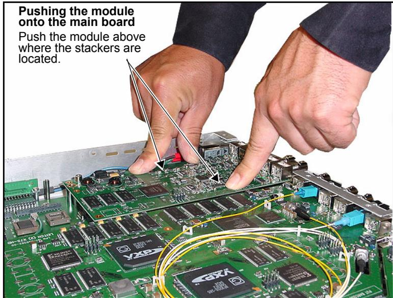
**Figure C-19.** Pushing the Module on to the Main Board
