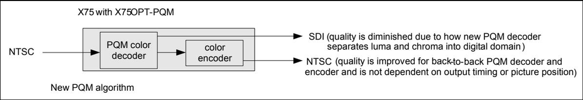
**Figure 3-8.** Alternate PQM Algorithm
