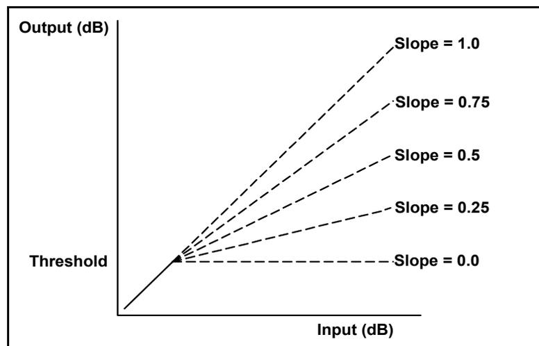
**Figure 3-4.** Audio Limiter Transfer Function
