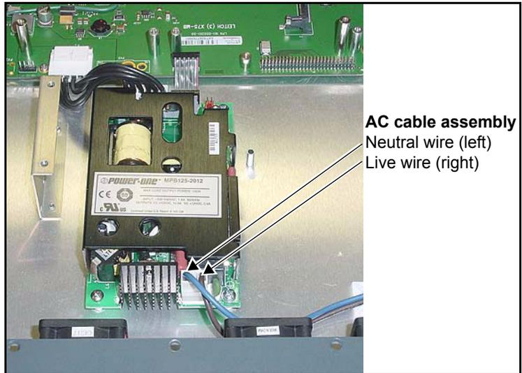
**Figure C-31.** Connecting AC Cables to Power Supply
