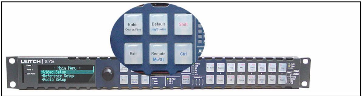
Figure 6-2. Control Knob and Menu Control Area
