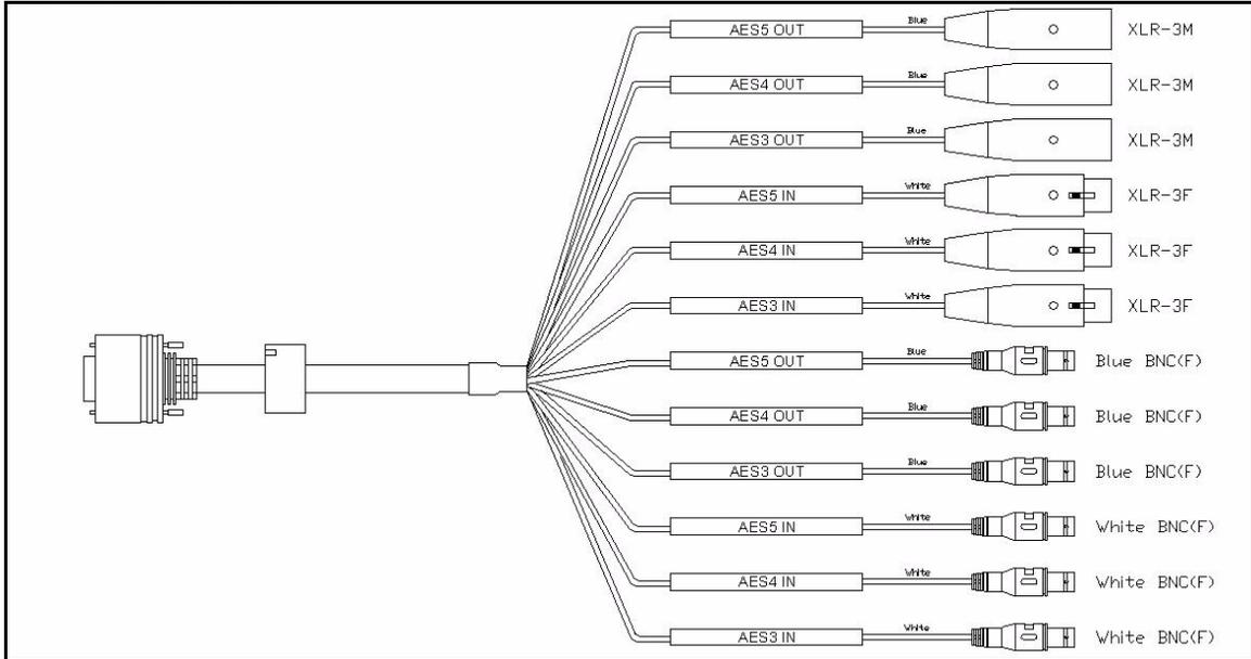
Figure A-11. CAB-X75HD-COMBO Cable Connectors
