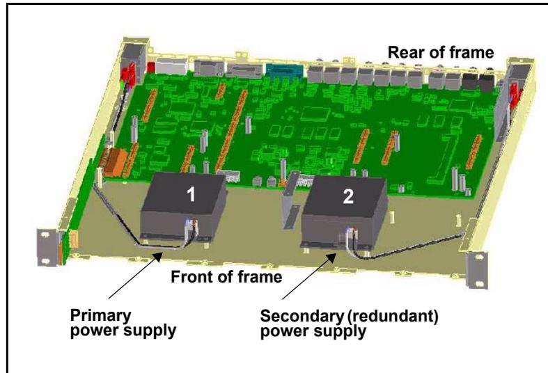
**Figure C-25.** Location of Connected Power Supply
