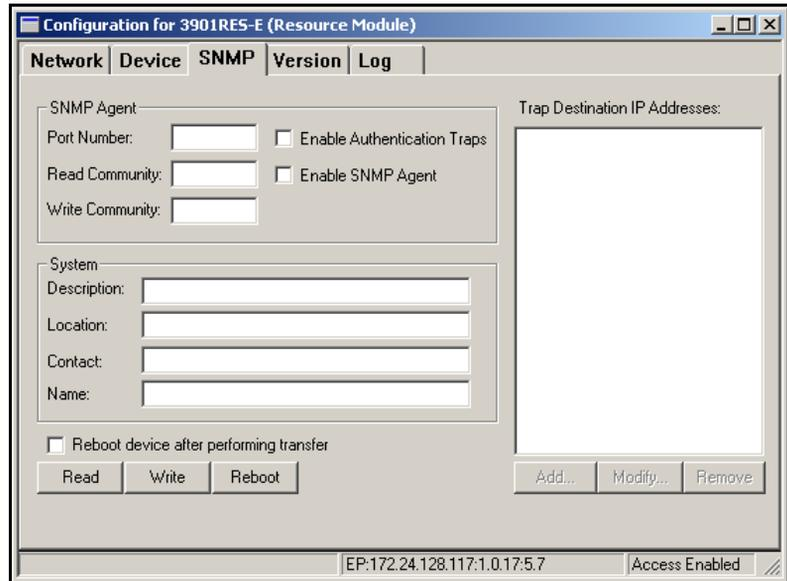
**Figure D-5.** SNMP Tab on device Configuration Window
