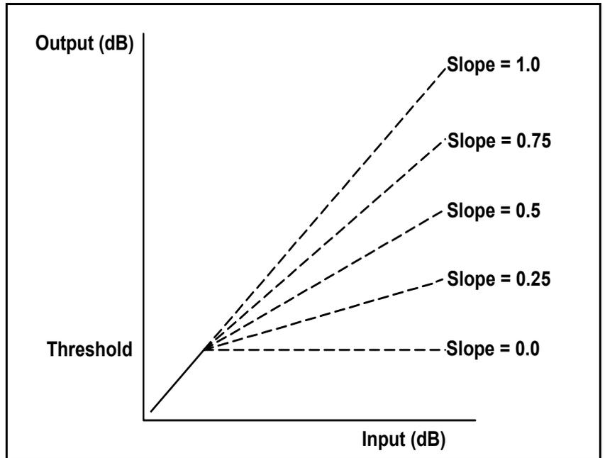
**Figure C-23.** Audio Limiter Transfer Function
