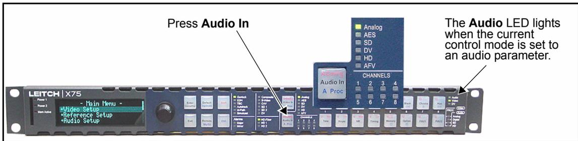
**Figure 9-1.** Audio Input Control Area
