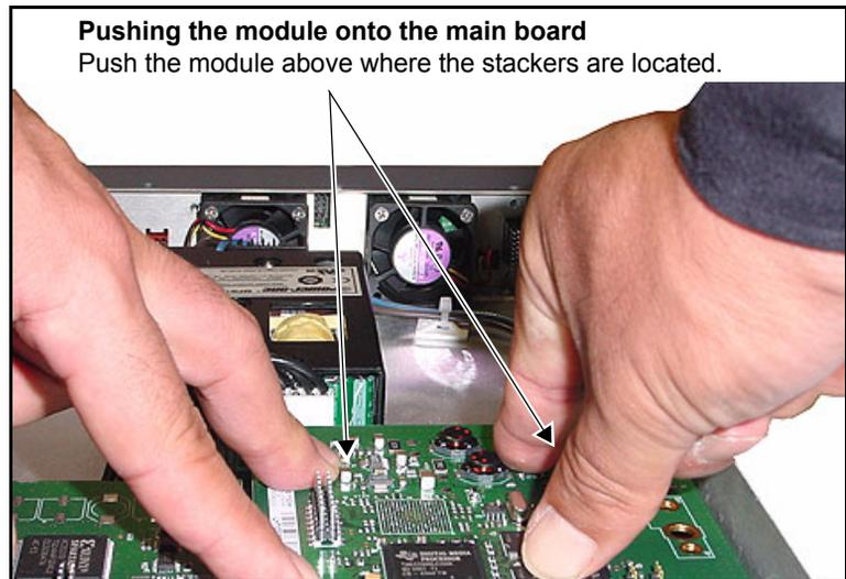
**Figure C-21.** Pushing the Module on to the Main Board
