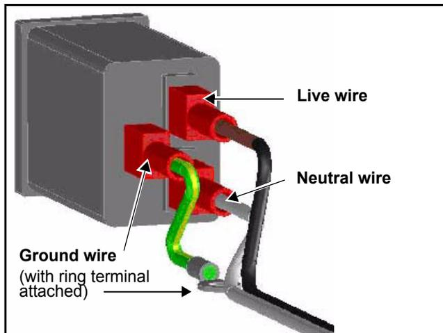
**Figure C-34.** Connecting AC Cables to Inlet
