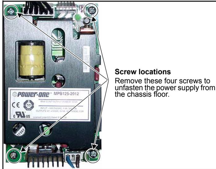
**Figure C-28.** Removing the Power Supply
