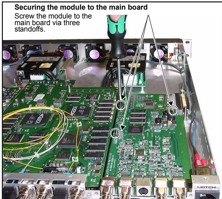
**Figure C-20.** Securing the Module to the Main Board
