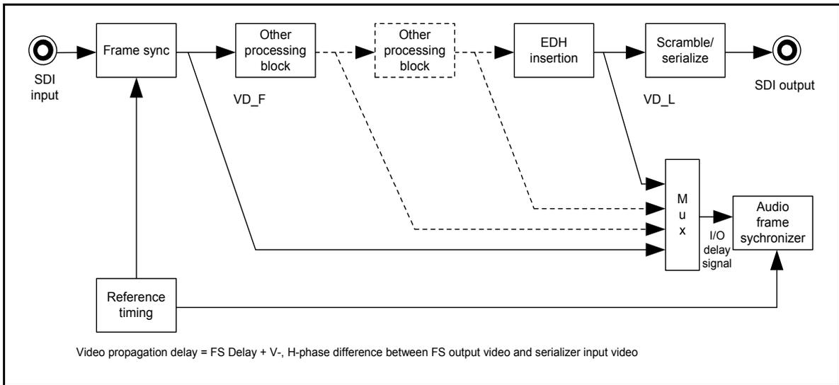
**Figure B-7.** I/O Delay Signal
