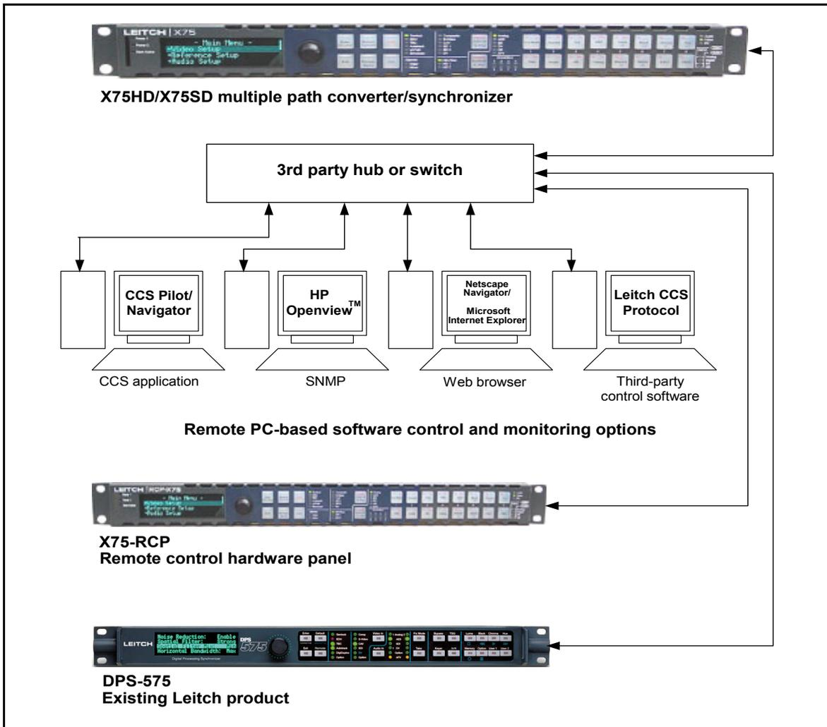
Figure 5-4. Network Configuration Diagram
