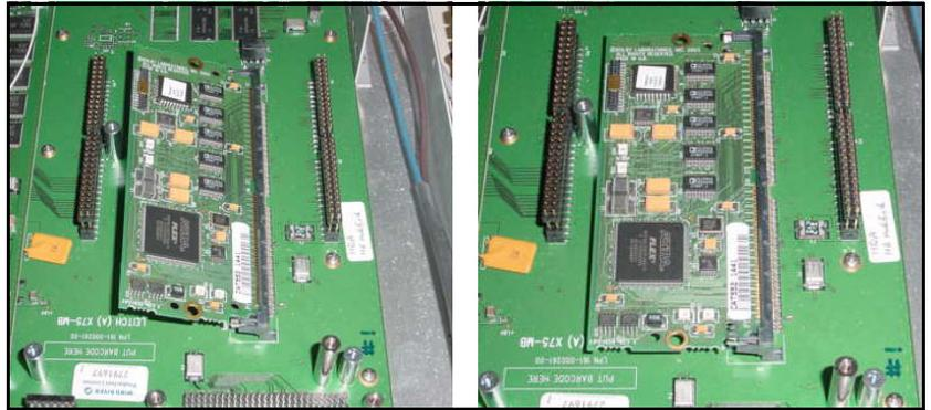
**Figure C-24.** Dolby Decoder Module Installation
