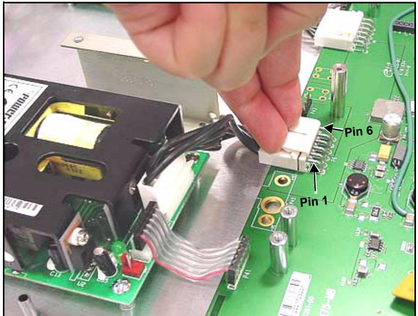
**Figure B-4.** Location of Power Supplies DC Cables
