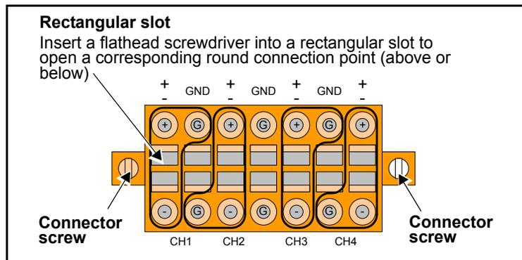
**Figure 3-3.** Installing Analog Audio Receptacles
