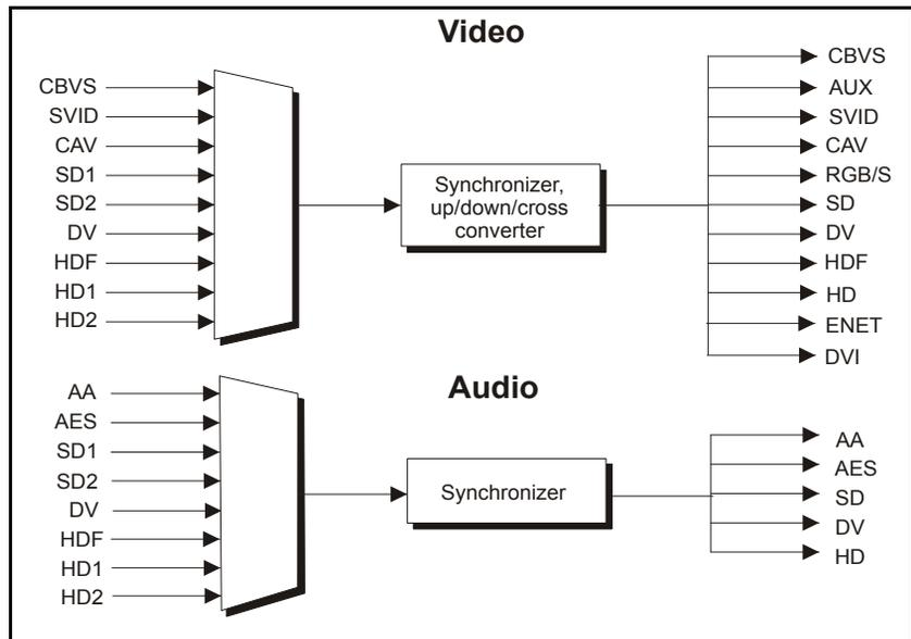
**Figure 1-6.** M-Path Single-Source Video and Audio Processing
