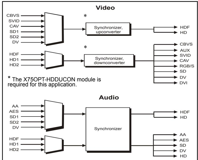
**Figure 1-7.** M-Path (Dual Source Video and Audio) Processing
