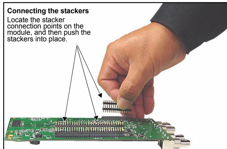
**Figure C-16.** Connecting Three Stackers to Module
