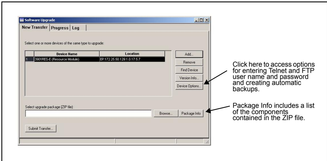
**Figure D-1.** Software Upgrade Tool's New Transfer Tab
