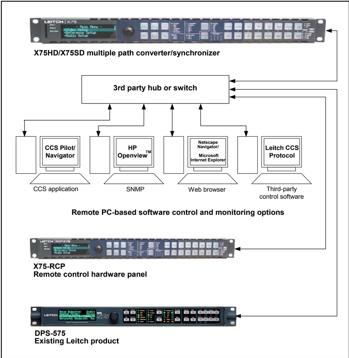
Figure 1-4. Typical Configuration, Control, and Monitoring Methods
