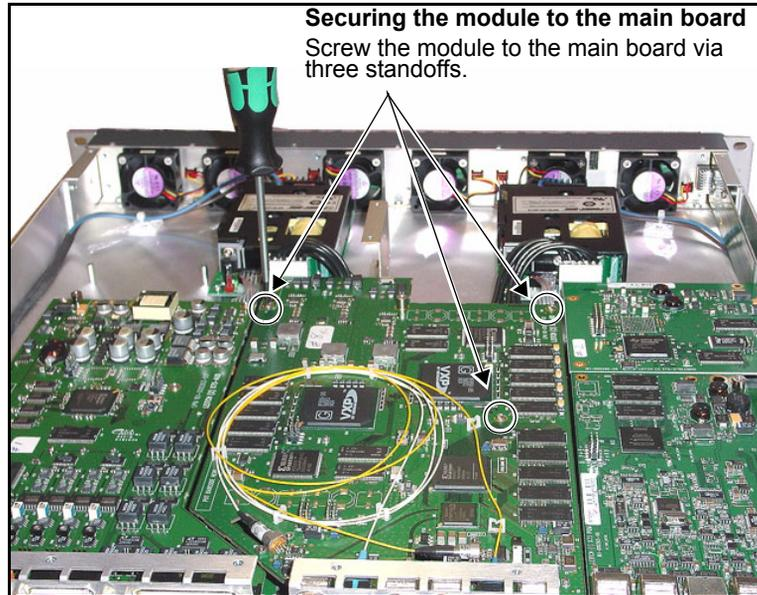
**Figure C-14.** Securing the Module to the Main Board
