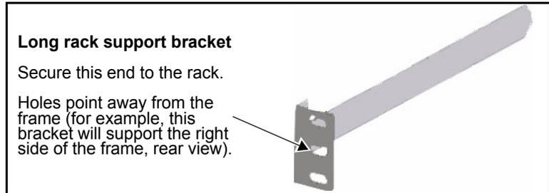
**Figure 4-4.** Long Rack Support Bracket
