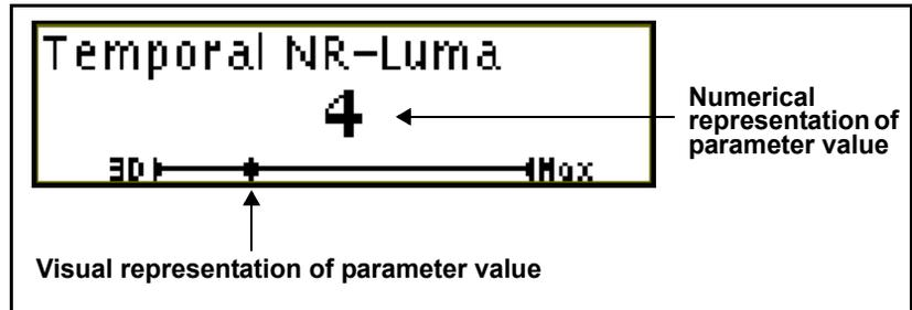
**Figure 6-3.** VFD Showing Numerical Range of Values
