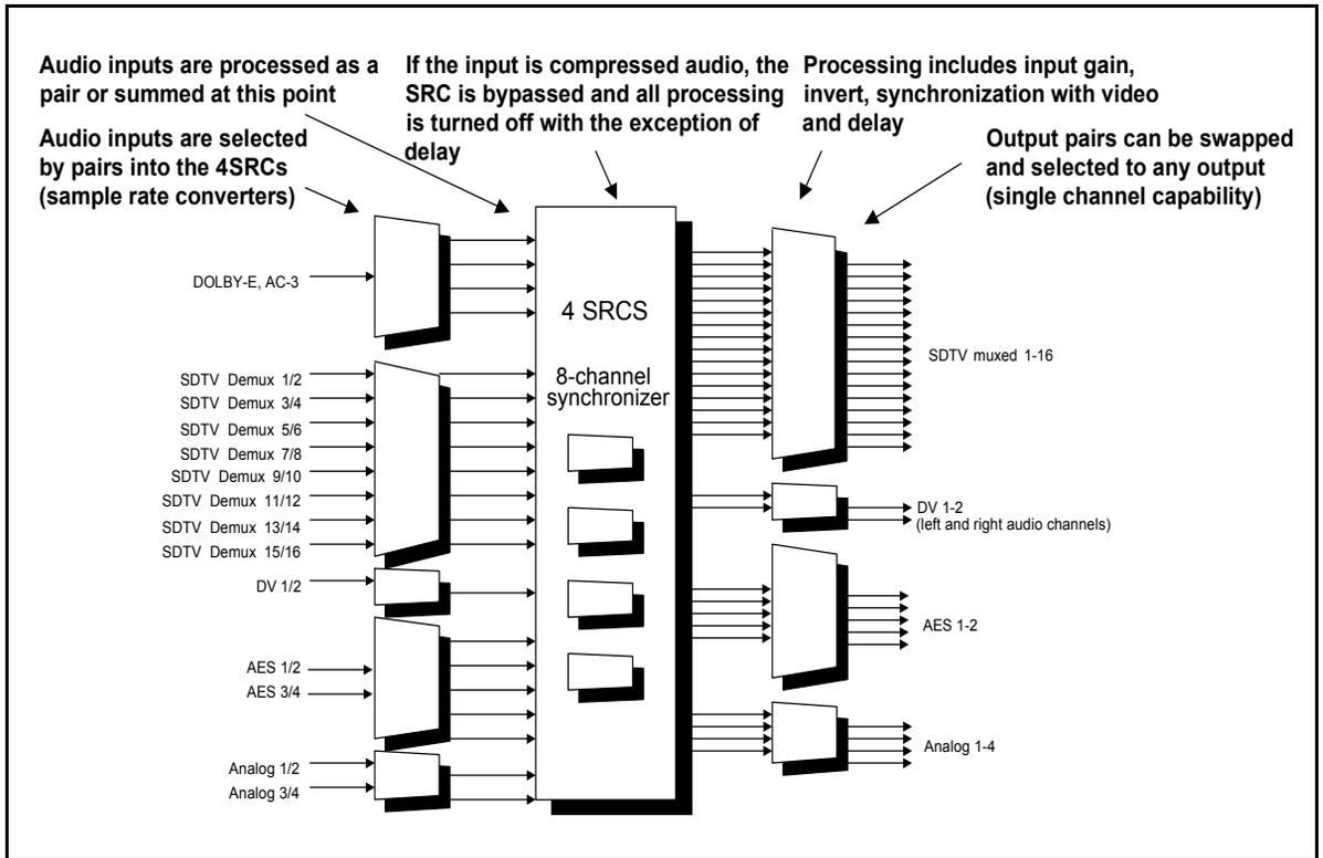
**Figure 1-9.** Audio Functional Block Diagram-8 Channel
