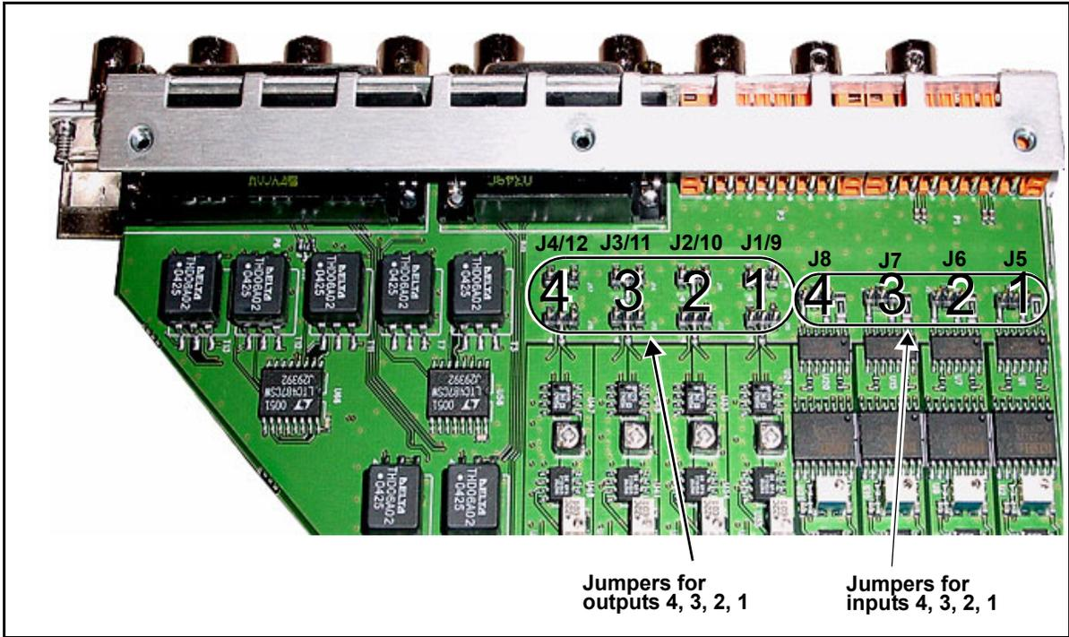
Figure 3-2. Jumper Locations for X75OPT-AS-16 and X75OPT-AS-8 Modules
