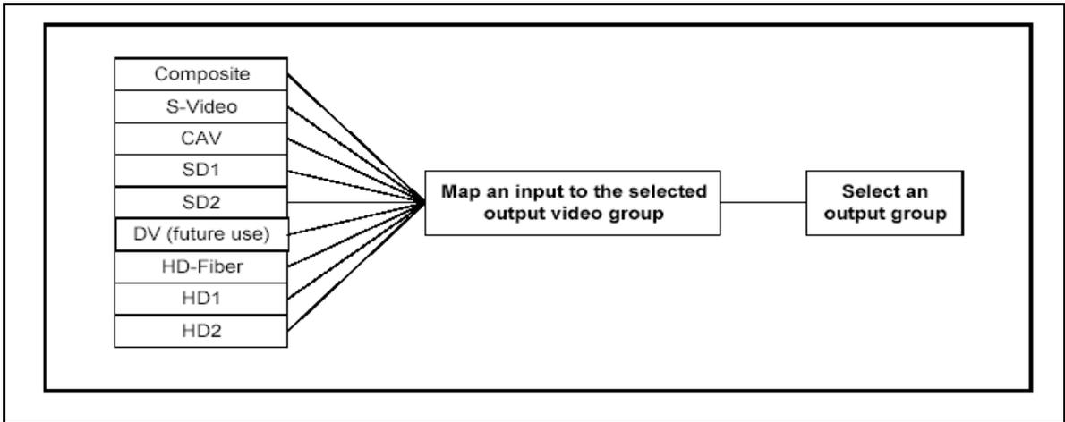
Figure 8-1. Single-Source Processing
