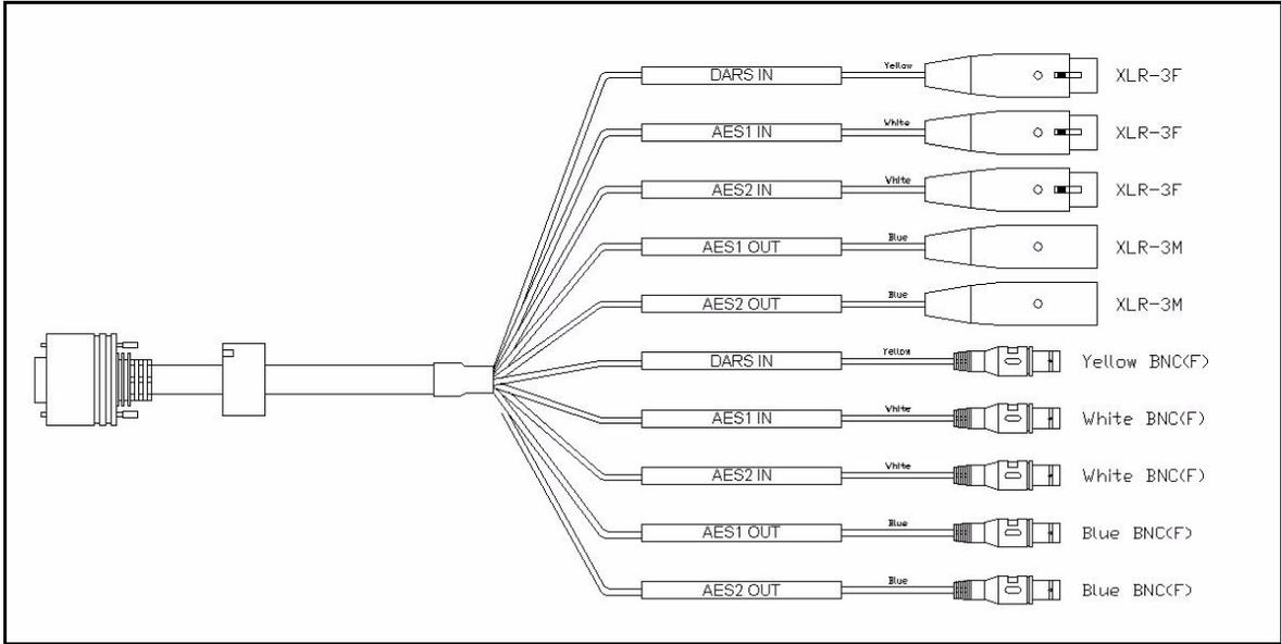
Figure A-9. X75OPTCAB-8-XC Cable Connectors
