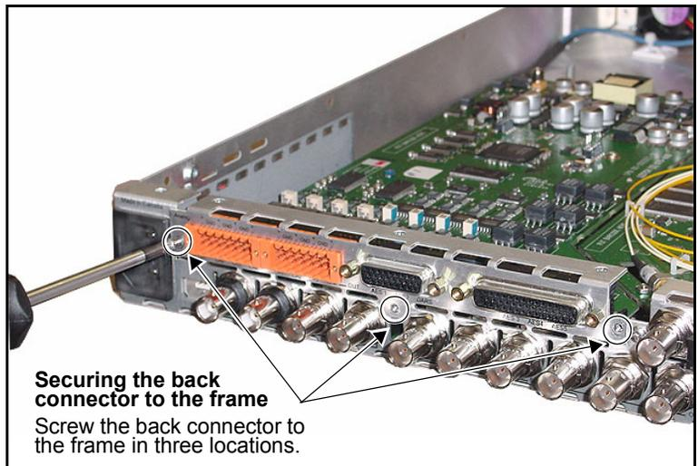
**Figure C-9.** Securing the Back Connector to the Frame
