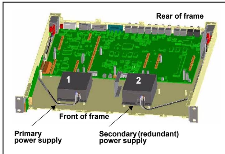
**Figure C-29.** Where to Install a Redundant Power Supply
