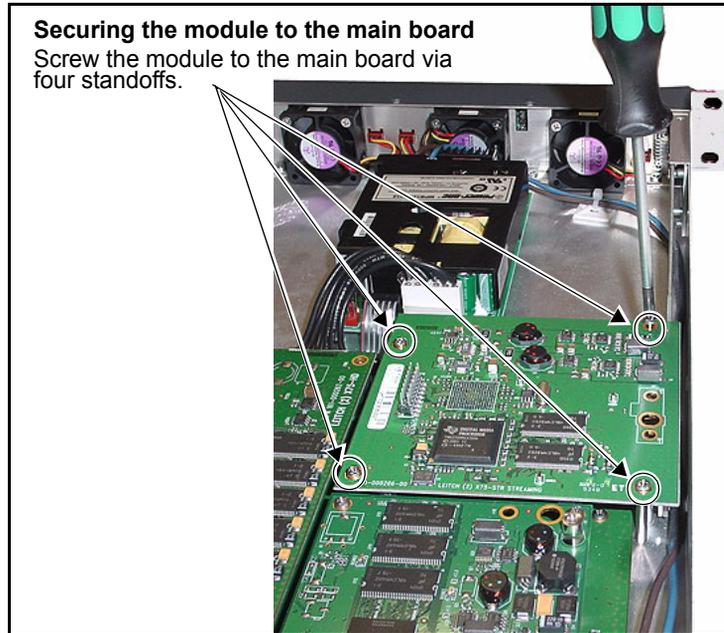
**Figure C-22.** Securing the Module to the Main Board
