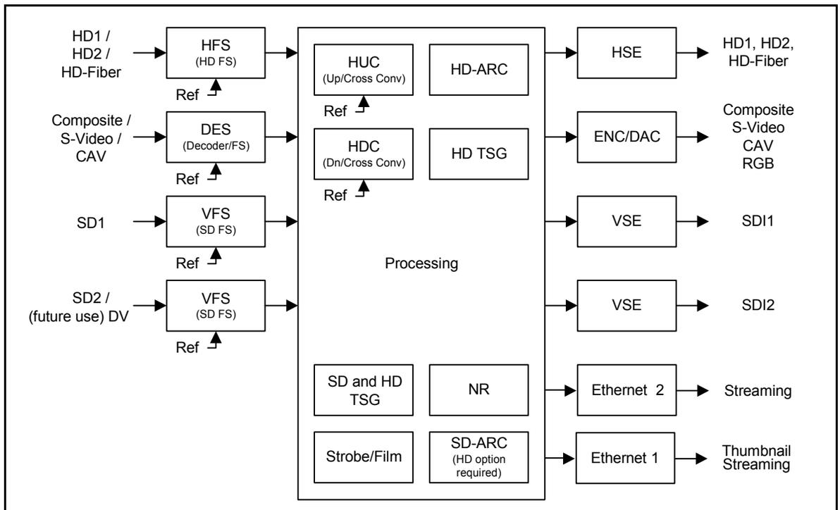
**Figure 1-5.** Video Functional Block Diagram
