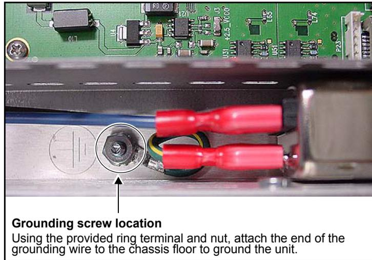
**Figure C-35.** Grounding AC Inlet
