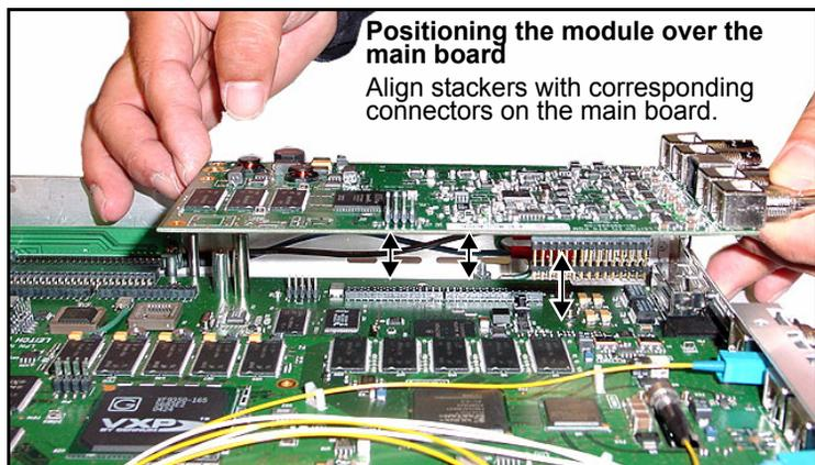
**Figure C-18.** Positioning Module over Standoffs
