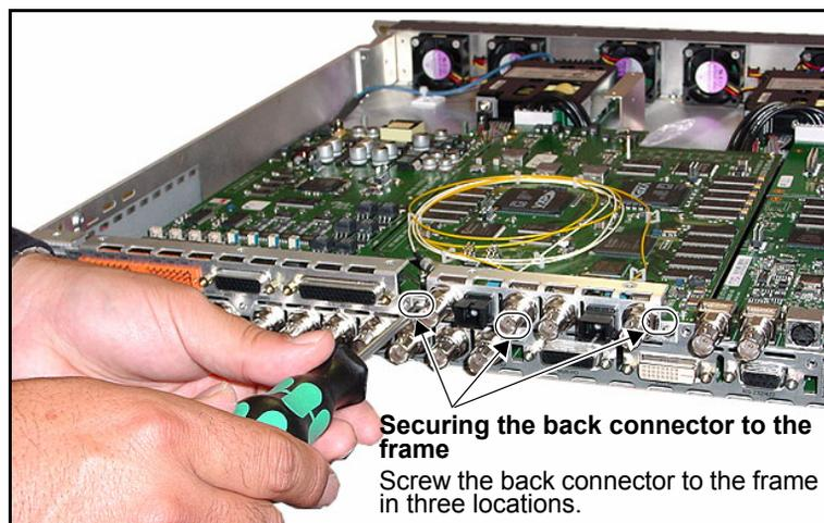
**Figure C-15.** Securing the Back Connector to the Frame
