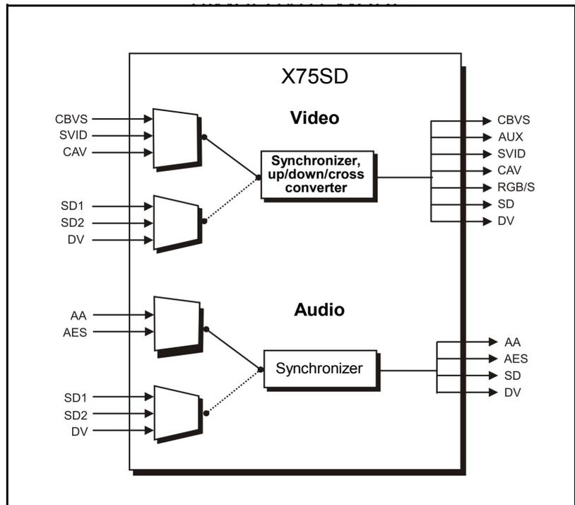
**Figure 1-11.** Simulcast Switcher Application
