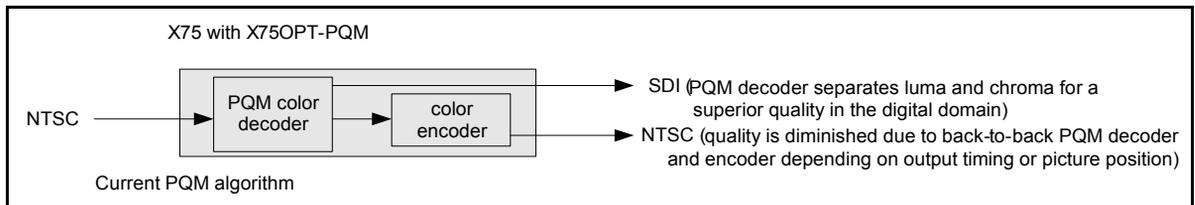
**Figure 3-7.** Current PQM Algorithm
