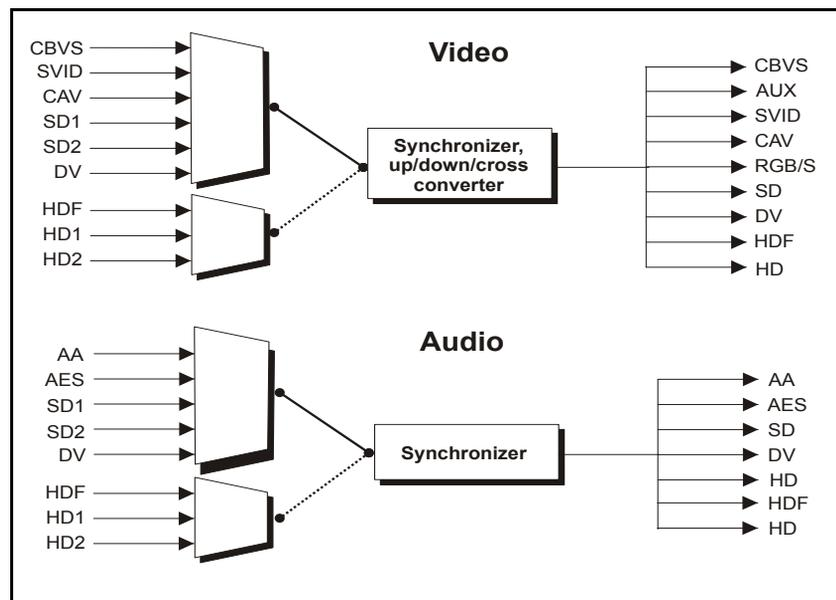
**Figure 1-10.** Simulcast Processing
