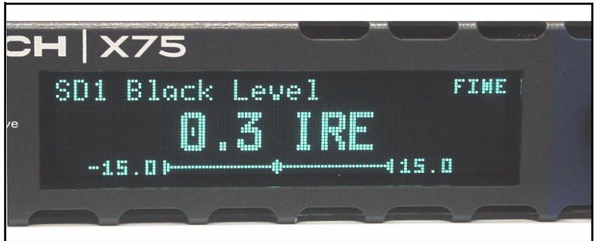
**Figure 2-3.** VFD Panel Showing Numeric Range of Values
