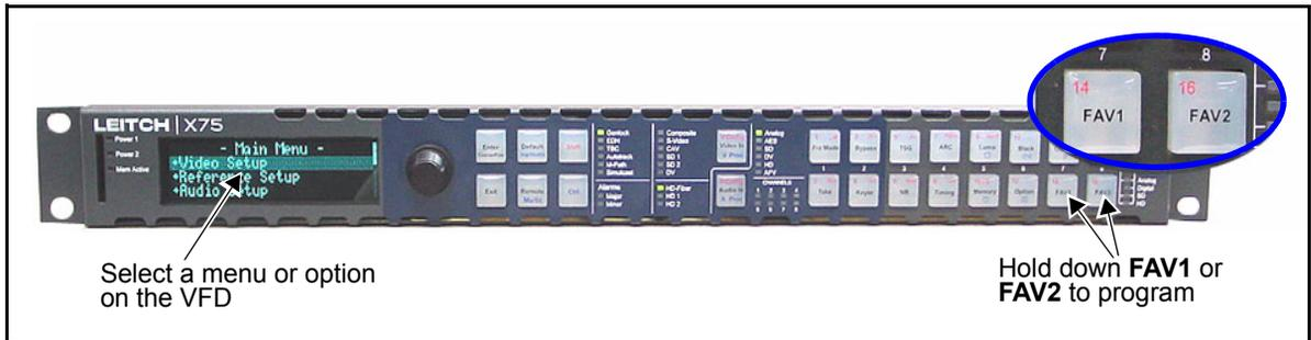
Figure 2-11. User-Programmable FAV1 and FAV2 Controls
