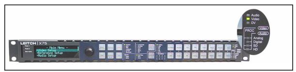
Figure 6-7. Control Mode Status LED Area
