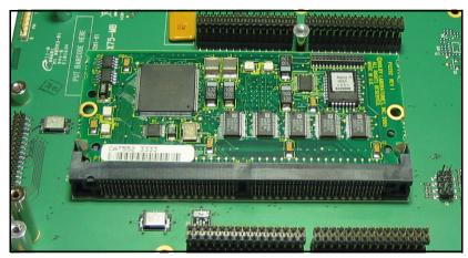
Figure C-27. Dolby Decoder Module Installed
