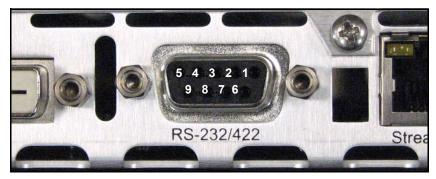
Figure 4. Data Port Pinouts
