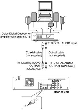
Note for connection: Remove the protection cap from the optical cable.
