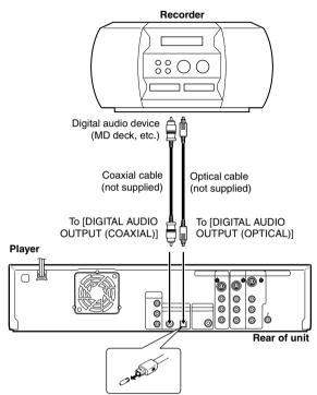
Note for connection: Remove the protection cap from the optical cable.
