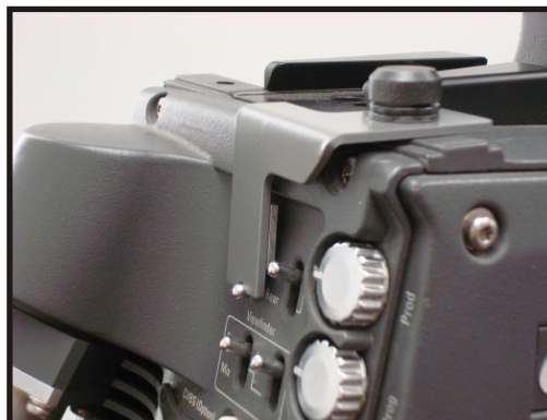
MST-1 Switch Retainer Installed on LDK back adaptor
